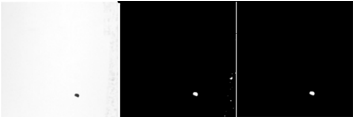
Figure 4. Sample frames from high-speed videos of the HDPE nurdles. MATLAB image processing tools are used isolate the nurdle numerically from the background creating black and white binary images at right with only the nurdle in frame.
