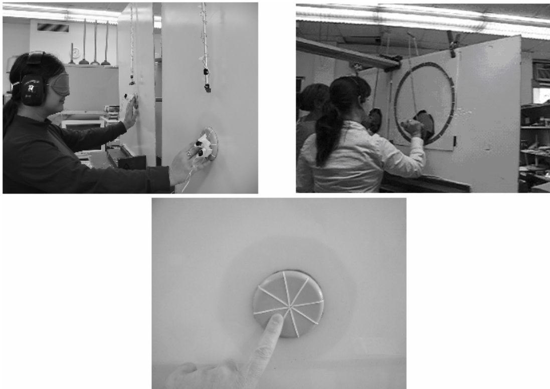
3: Setup for Experiment 2. Top panel: Two drivers moving paddles in a square template (left) and in a circular template (right). Curtain between experimenters removed for this photo. Middle panel: A participant haptically tracking the two magnetically driven target buttons. Bottom panel: Target button and participant's index finger without IREDS attached.
