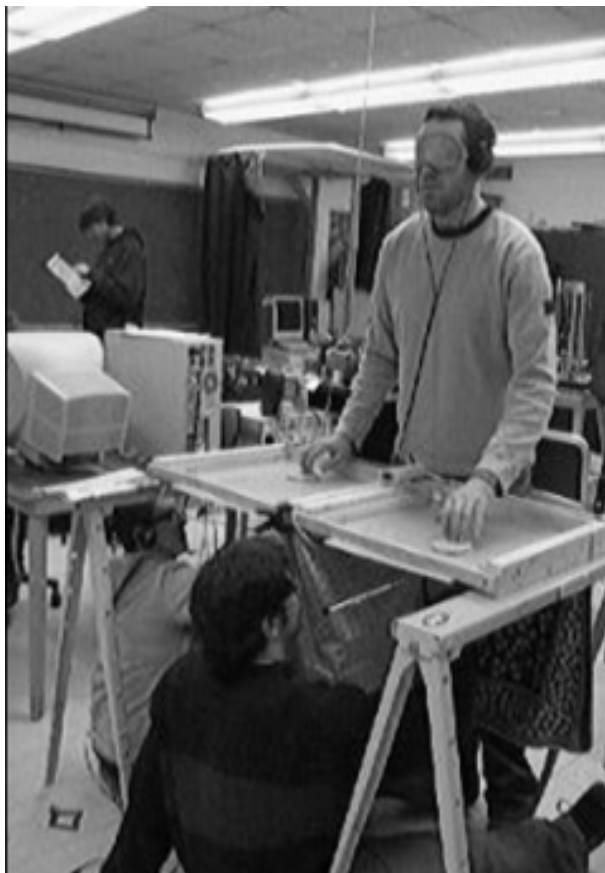
5: The setup for Experiment 4. Two drivers under the tabletop moved the paddles connected to magnetized targets while the subject haptically tracked the targets. The driver on the far left side of the picture abruptly changed directions according to a computerized tone that only she could hear.
