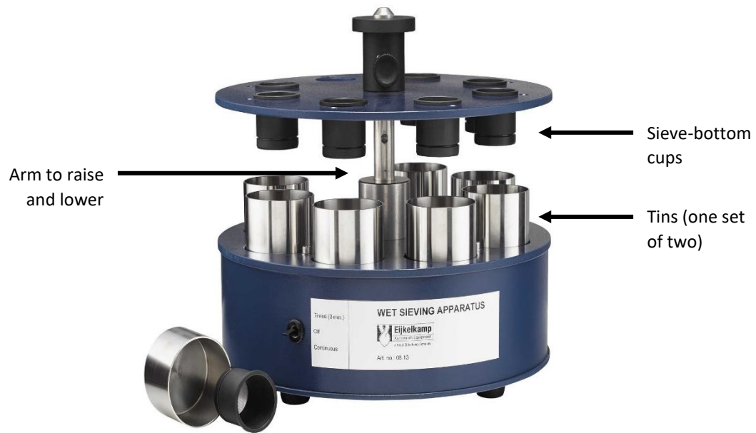
Figure 2.3. Wet sieving apparatus (Eijkelkamp Soil & Water Giesbeek, Netherlands) used to measure water stable aggregates.
