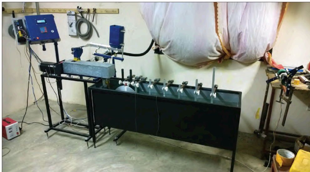
Figure 2.3: Thunderhead filament extruder prototype in Tanzania
