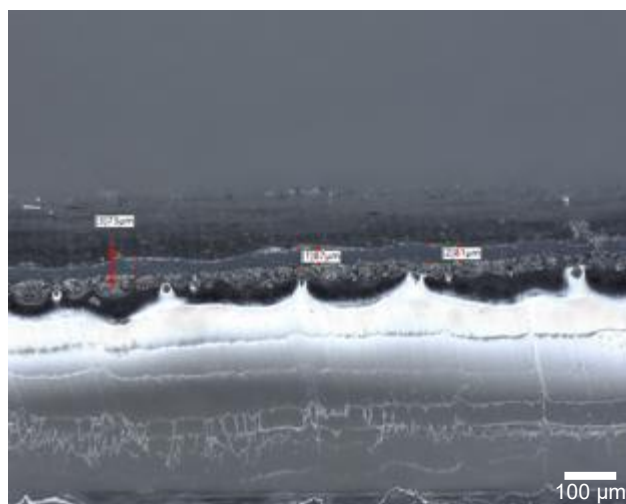
Figure 3-5: Thickness of spin-coated PDMS on top of transferred LIG.
