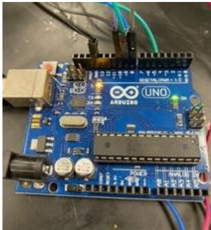
Figure A-7: Arduino board configuration for controlling the linear stage.
