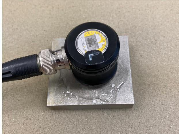
Figure 4-5: Example of transducer orientation for pulse-echo testing on top of a foam block.
