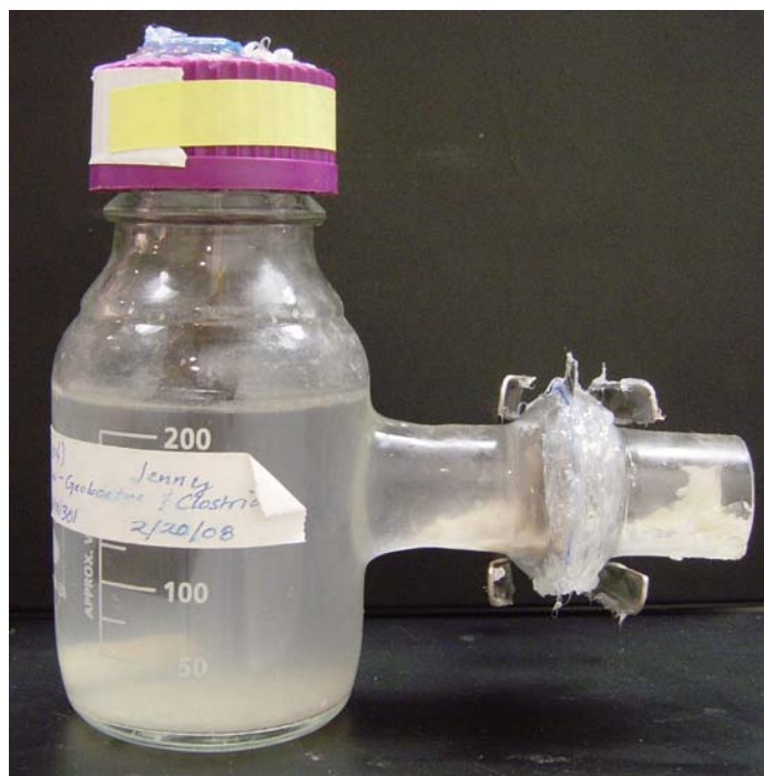
Figure 3-1: Bottle MFC reactor used in these experiments
