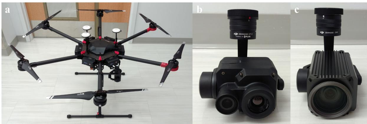
**Figure 1.** Hardware components employed in the study: (a) unmanned aerial vehicle (UAV), (b) thermal camera, and (c) red green blue (RGB) camera.
