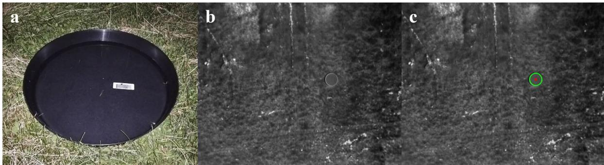
**Figure 5.** A ground control point (GCP) for georeferencing thermal mosaics: (a) in the orchard, (b) its appearance in a thermal image, and (c) being detected by the algorithm.
