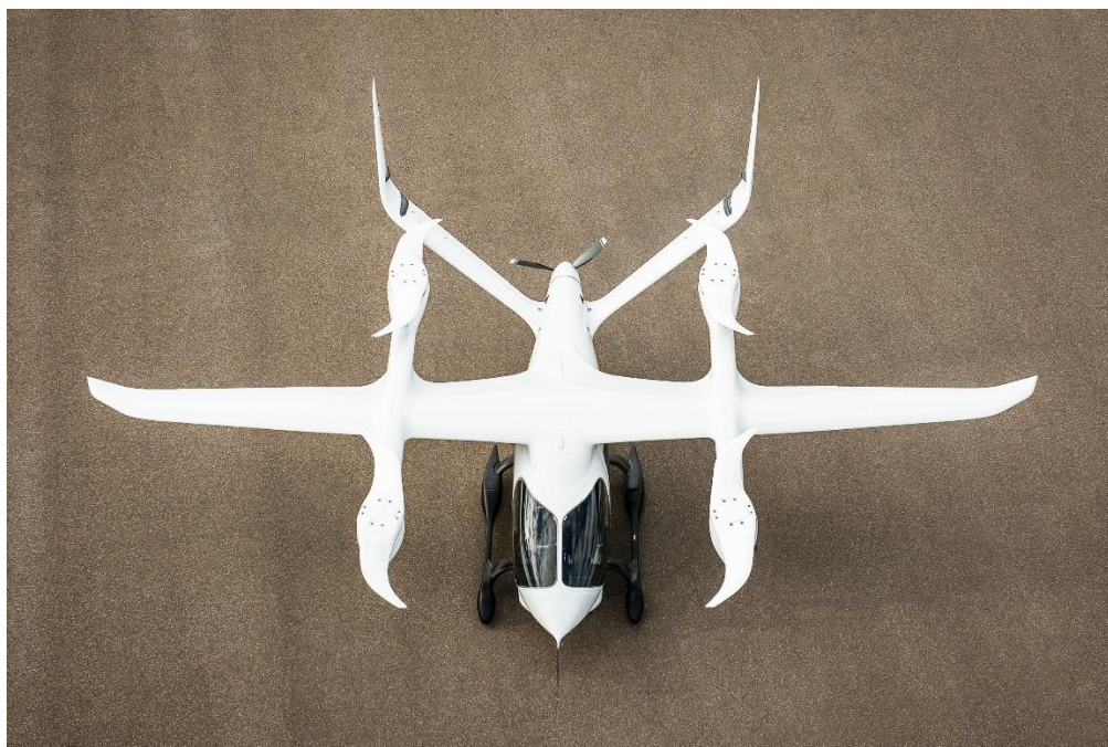
Figure 4.1 Latest BETA Alia aircraft with larger rotor blades for the lift rotors (downloaded from beta.team).
