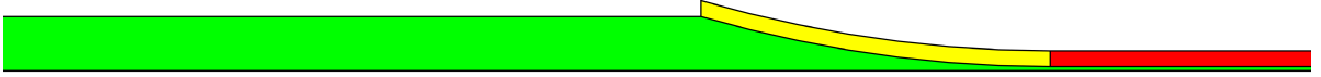
Figure A.1. Graphical depiction (not to scale) of the test geometry whose material parameters and dimensions are given in Table A.1. Green denotes the beam material, yellow denotes the Damping 1 material, and orange denotes the Damping 2 material.
