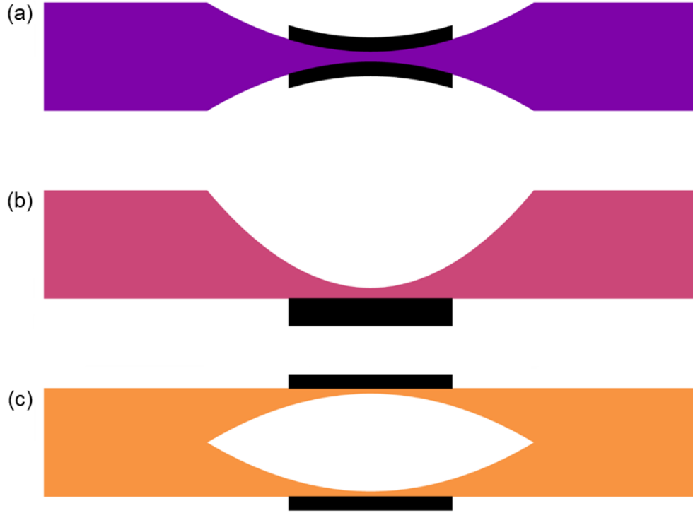
Figure 4.1. Three styles of one-dimensional acoustic black hole vibration absorbers (not to scale). The three styles are (a) Standard symmetric; (b) Standard nonsymmetric; and (c) Double-leaf. Added damping is indicated in black. Note that the colors used for each style in this figure will be used throughout the chapter to indicate each color’s respective style.
