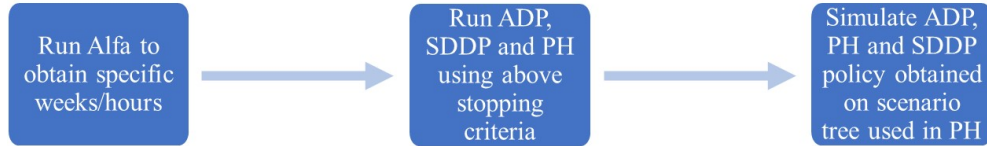
Figure 4.1: Analysis flowchart: Sample 3000 investments and uncertainties and run the alfa algorithm to obtain the specific hours/weeks for each problem. After obtaining these weeks, run ADP, SDDP and PH using these weeks to obtain a policy. Simulate this policy on the same scenario tree as PH to obtain the simulated cost.
