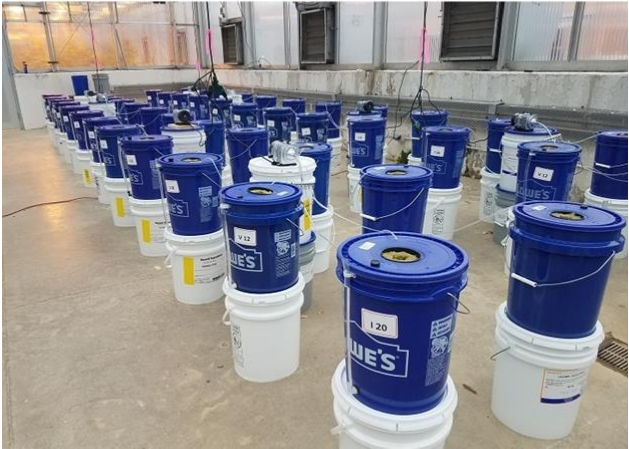
Figure 5.2: Buckets used as experimental units. Visible are the airlines, seated 76mm rockwool blocks in net pots, and standpipes. View is down a block (I20, V12, etc..) placed perpendicular to the airflow from cooling fans seen in background.
