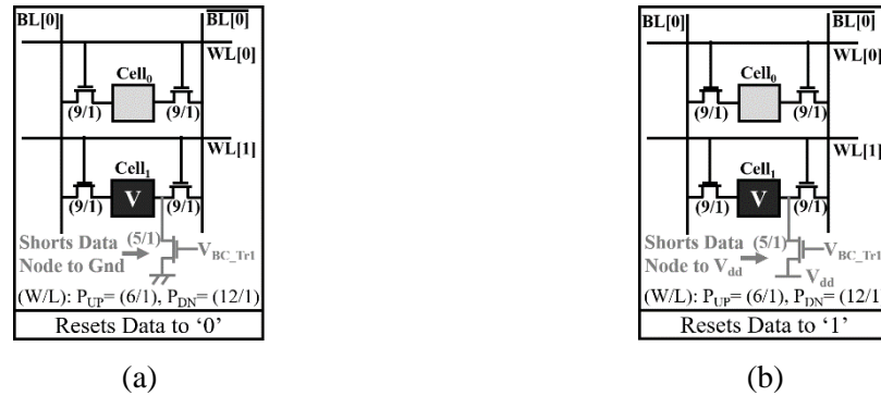
Figure 5-4: TLB entry reset to (a) 0; and (b) 1. The sizes of SRAM pull-up, pull-down and access transistors are shown. The back-to-back inverters in SRAM are omitted for clarity.
