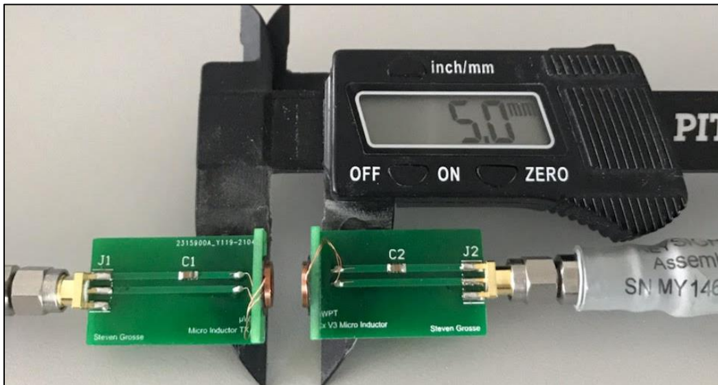
Figure 4.9: Experimental setup setting separation distance at g = 5.0 mm
