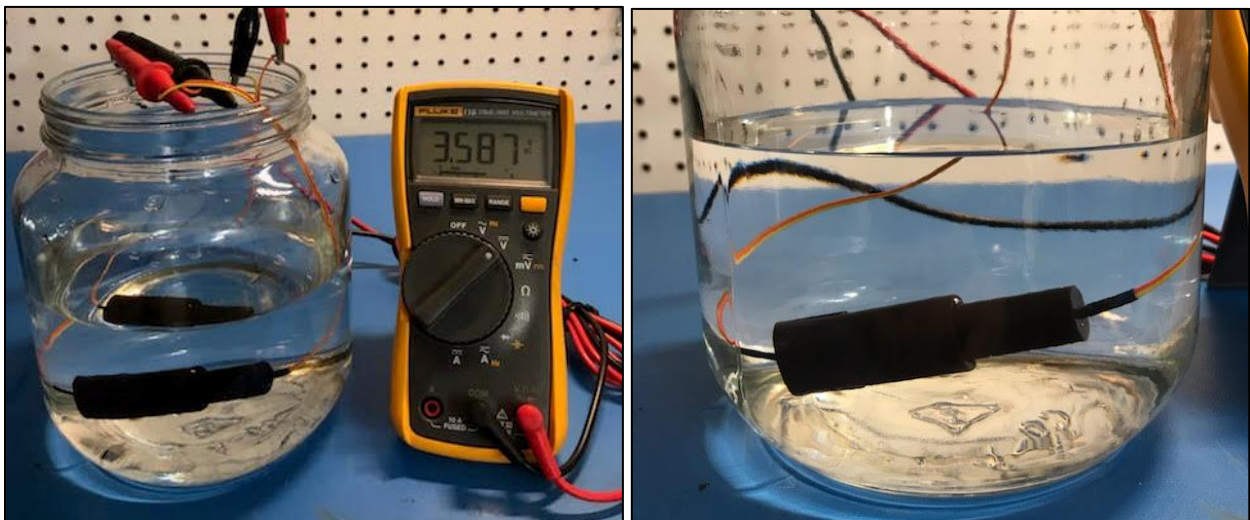
Figure 5.13: NMC prototype submerged under water with no water contamination
