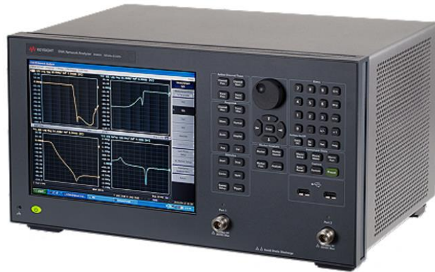
Figure 4.4: Keysight VNA E5063A used for experimental measurements
