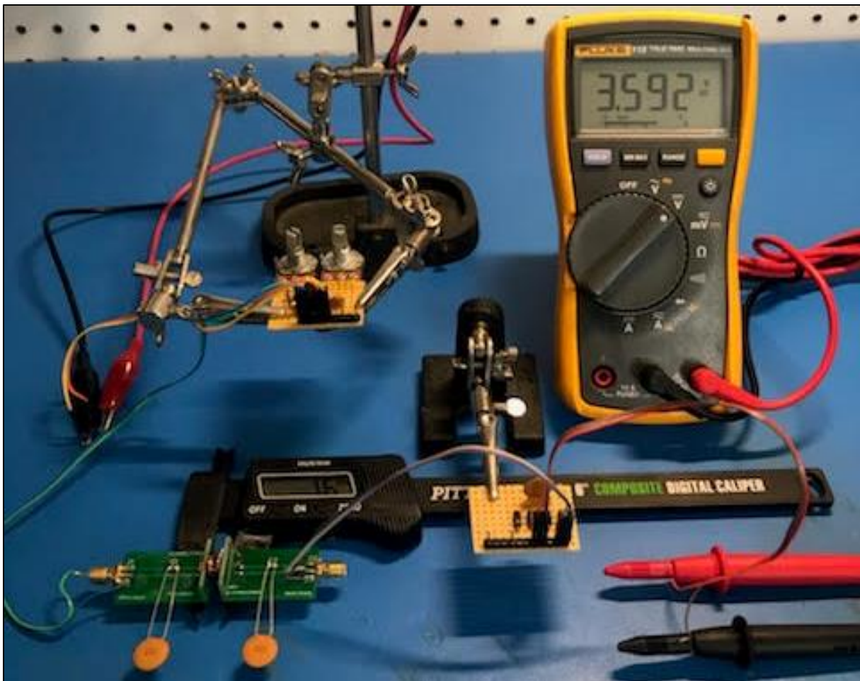
Figure 5.9: Experimental setup connected to a DMM for a DC voltage measurement
