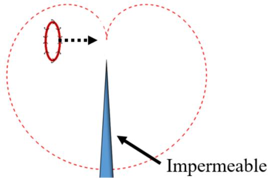
Figure 2.4: Cardioid sound directivity from a vortex ring convecting near an impermeable non-compact plate
