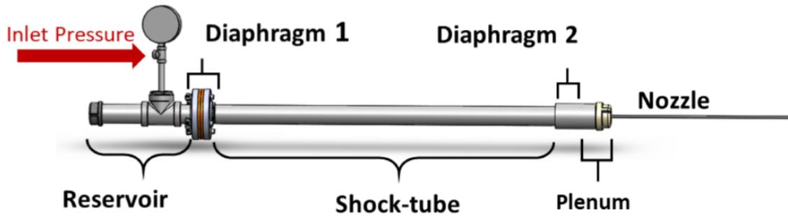
Figure 3.2: A CAD model of the vortex ring generator with the primary components labeled.
