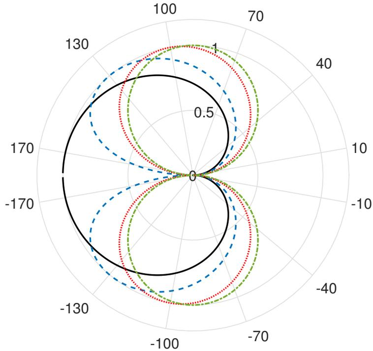
Figure 3.7: Predicted changes in acoustic radiation directivity with plate porosity at each plate listed in Table 3.2. Here, the solid (—) refers to  $\mu/k = 0$ , (---)  $\mu/k = 0.49$ , (· · ·)  $\mu/k = 3.10$ , and (-·-)  $\mu/k = 58.9$ .
