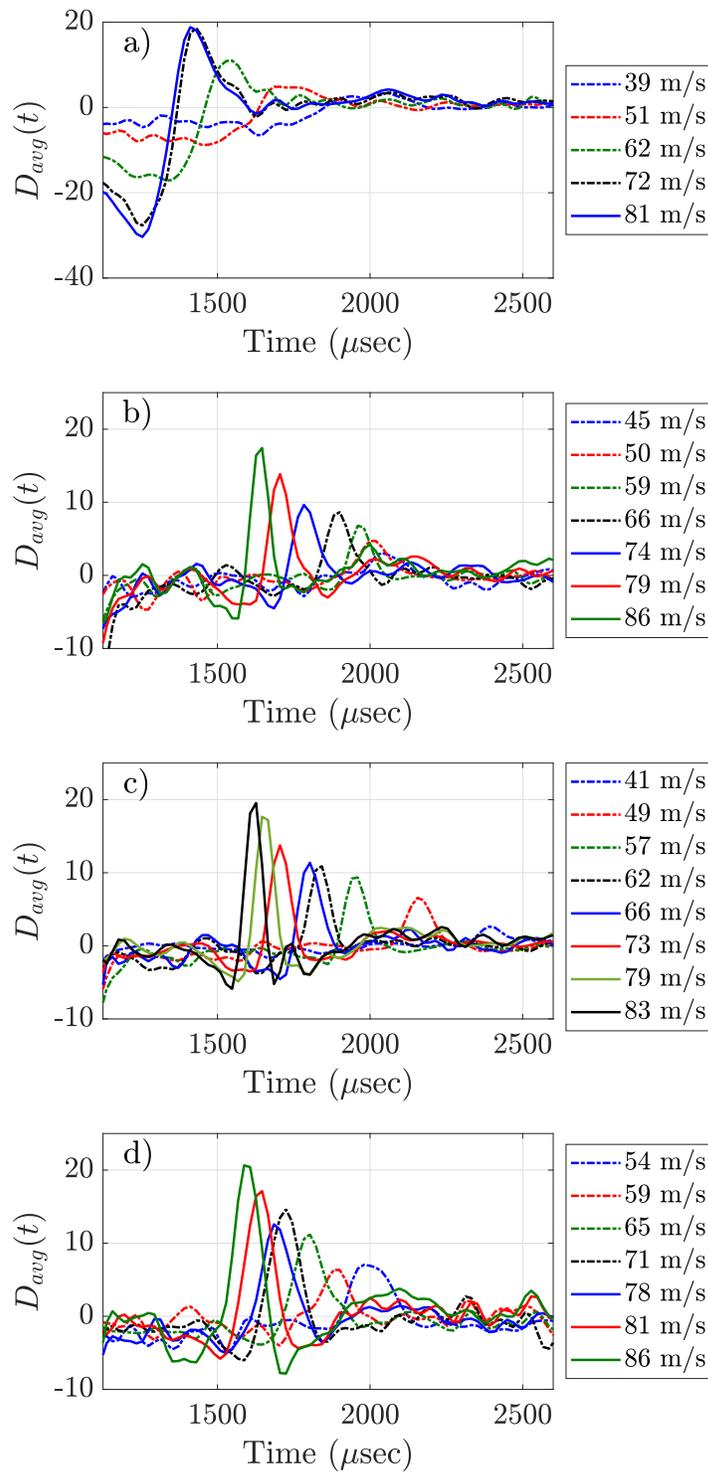
Figure 4.6: Averaged source waveforms,  $D_{t_{avg}}(t)$ , for (a)  $\mu/k = 0$ , (b)  $\mu/k = 0.49$ , (c)  $\mu/k = 3.10$ , and (d)  $\mu/k = 58.9$ . Line color and type indicate vortex ring speed shown in legends.
