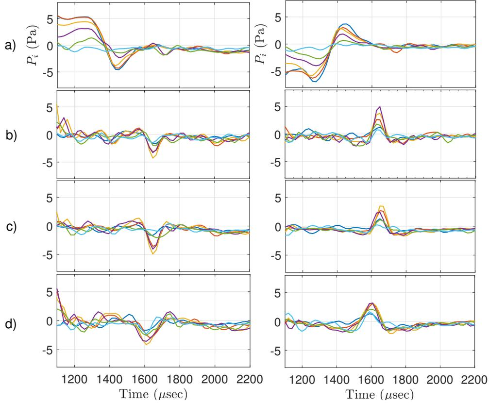
Figure 4.2: Sound pressure waveforms  $p_i(\theta)$  for (a)  $\mu/k = 0$ , 81 m/s, (b)  $\mu/k = 0.49$ , 86 m/s, (c)  $\mu/k = 3.10$ , 79 m/s, and (d)  $\mu/k = 58.9$ , 86 m/s. Right column:  $\theta > 0$ , left column  $\theta < 0$ ,  $-\pm 170^\circ$ ,  $-\pm 130^\circ$ ,  $-\pm 100^\circ$ ,  $-\pm 70^\circ$ ,  $-\pm 40^\circ$ ,  $-\pm 10^\circ$ .
