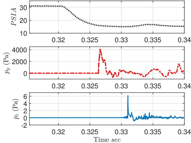
Figure 3.10: Overview of time series of events observed by the reservoir pressure gage (top), plenum pressure transducer (middle), and a radial microphone ( $\theta = -170, r = 500\text{mm}$ ) (bottom)
