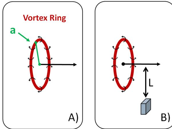
Figure 2.2: Schematic of compact acoustic source, in the form of a vortex ring A) convecting in free space and B) near a compact body
