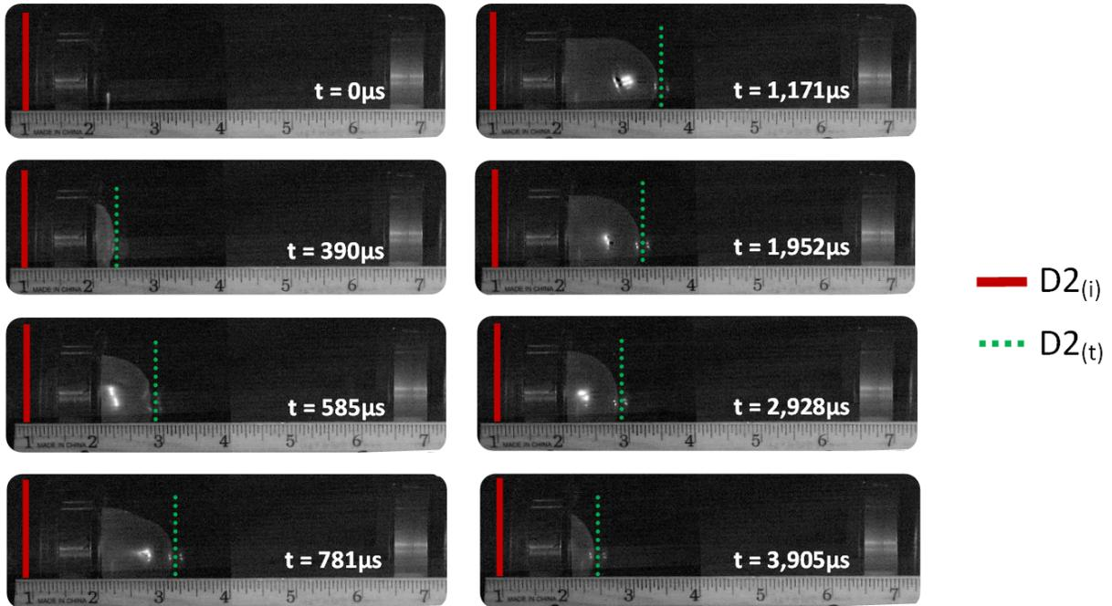
Figure 3.5: Time laps deformation of diaphragm D2 due to collision with shock wave.  $D2_i$  is the resting position, and  $D2_t$  is the maximum deformation for each time stamp.
