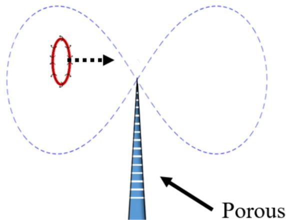
Figure 2.5: Acoustic dipole directivity from a vortex ring convecting near the edge of a non-compact rigid porous plate
