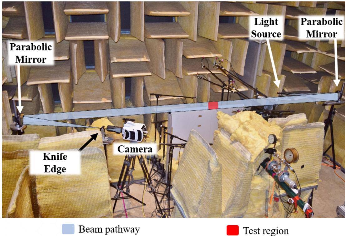
Figure 3.8: Z-configuration Schlieren setup within the anechoic chamber where the blue-gray overlay shows the optical path.
