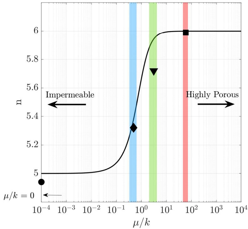
Figure 4.4: Comparison of predicted values of sound power law exponent  $\bar{n}$  to measurement. The shaded regions blue, green, and red represent the  $\mu/k$  ranges for  $\mu/k = 0.49$ ,  $\mu/k = 3.10$ , and  $\mu/k = 58.9$ , respectively. The symbols indicate a)  $\circ$   $\mu/k = 0$  and  $\bar{n} = 4.94$ , b)  $\diamond$   $\mu/k = 0.49$  and  $\bar{n} = 5.32$ , c)  $\nabla$   $\mu/k = 3.10$  and  $\bar{n} = 5.70$ , and d)  $\square$   $\mu/k = 58.9$  and  $\bar{n} = 5.99$ .
