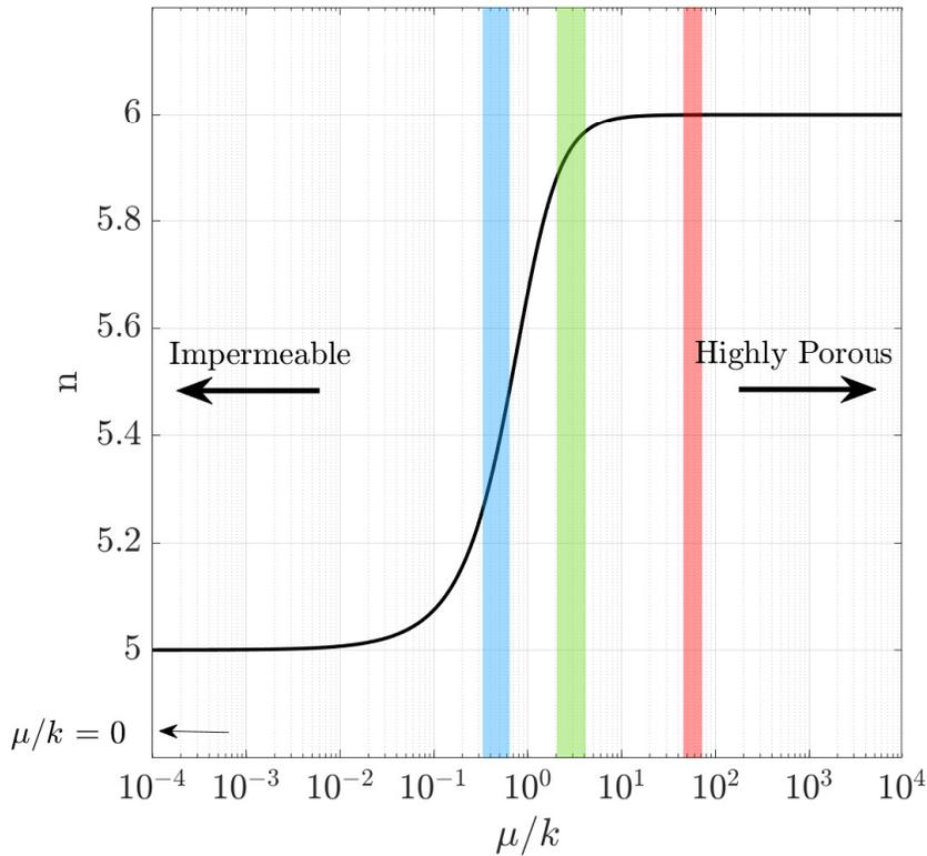
Figure 3.6: Predicted changes in acoustic radiation with plate porosity for power law exponent,  $n$ . Colored bands indicate approximate ranges of porosity for the plates listed in Table 3.2.
