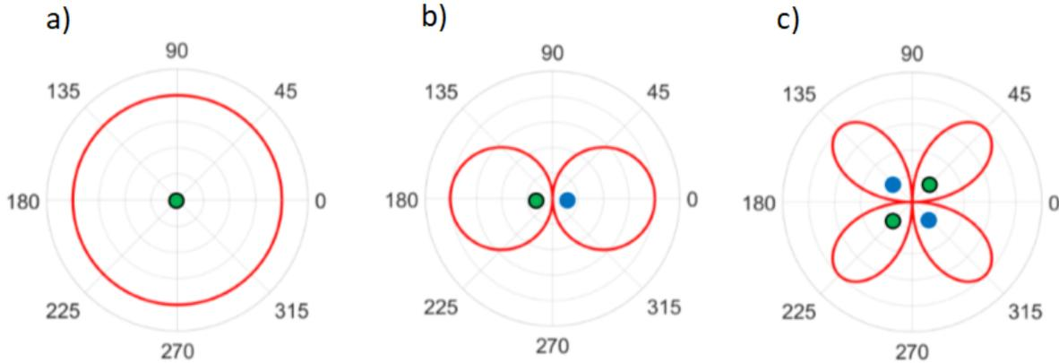
Figure 2.1: Radiated sound directivity, shown as a  $(-)$ , for a) monopole, b) dipole, and c) quadrupole sources.
