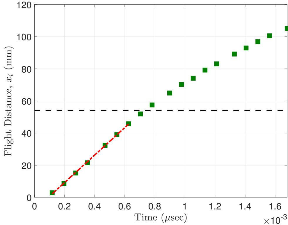
Figure 3.13: Vortex ring speed ( $U_R$ ) determined from the high speed Schlieren image analysis.  $\square$  indicate the mean vortex ring location ( $x_i$ ) at time step ( $t$ ),  $(- -)$  the linear fit to determine ( $U_R$ ), and the horizontal dashed line  $(- -)$  is the edge location. For this realization  $U_R$  is 83 m/s,  $Z_p = 56$  mm and  $\mu/k = 3.10$ .
