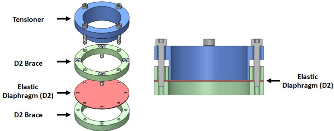
Figure 3.4: An exploded and sectional view CAD drawing of the diaphragm tension device.
