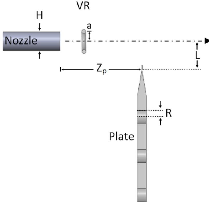
Figure 1.2: Trailing edge noise problem modeled as a vortex ring passing near an edge of a porous plate. Here,  $H$  is the nozzle diameter,  $L$  impact distance,  $Z_p$  offset between the nozzle and edge,  $a$  vortex ring radius,  $R$  the radius of the hole, and VR the vortex ring convecting at speed  $U$ .
