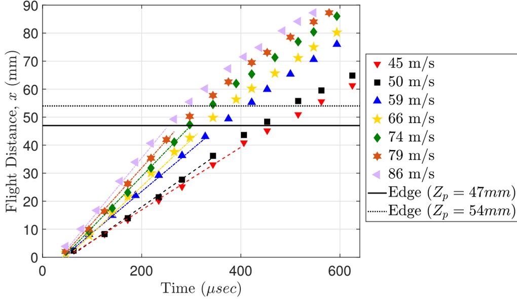
Figure 4.1: Vortex ring motion for different ring speeds for  $\mu/k = 0.49$  at fixed  $L = 9.8\text{mm}$ . Vortex ring position ( $x$ ) vs time. Data points obtained from high-speed video analysis. Dot-dashed lines (-.) indicate linear fits up to dotted line (:)  $Z_p = 54\text{mm}$ . Dashed lines (--) indicate linear fits up to solid line (-)  $Z_p = 47\text{mm}$ . The slope of the dot-dashed (-.) and dashed (--) lines provides an estimate of ring approach speed,  $U_R$ .
