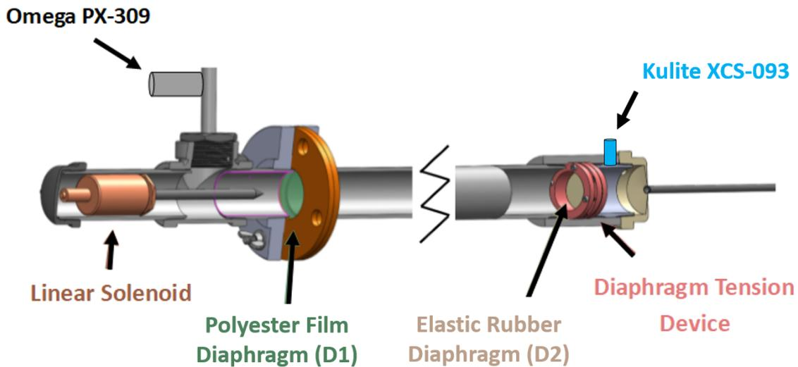
Figure 3.3: A CAD model of the vortex ring generator with the primary components labeled.
