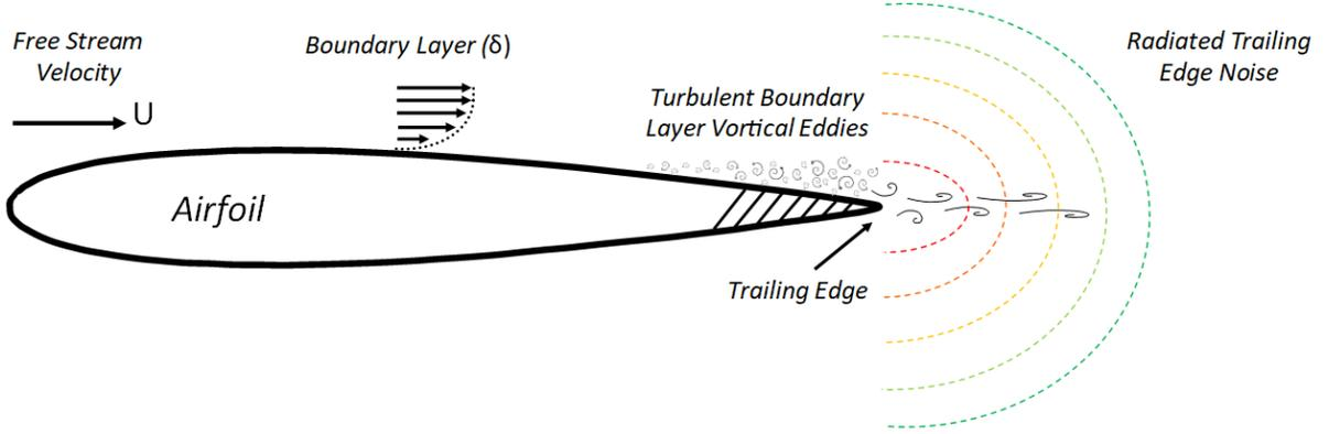
Figure 1.1: Schematic of the turbulent boundary, formed on a single side of the airfoil for clarity, and trailing edge noise
