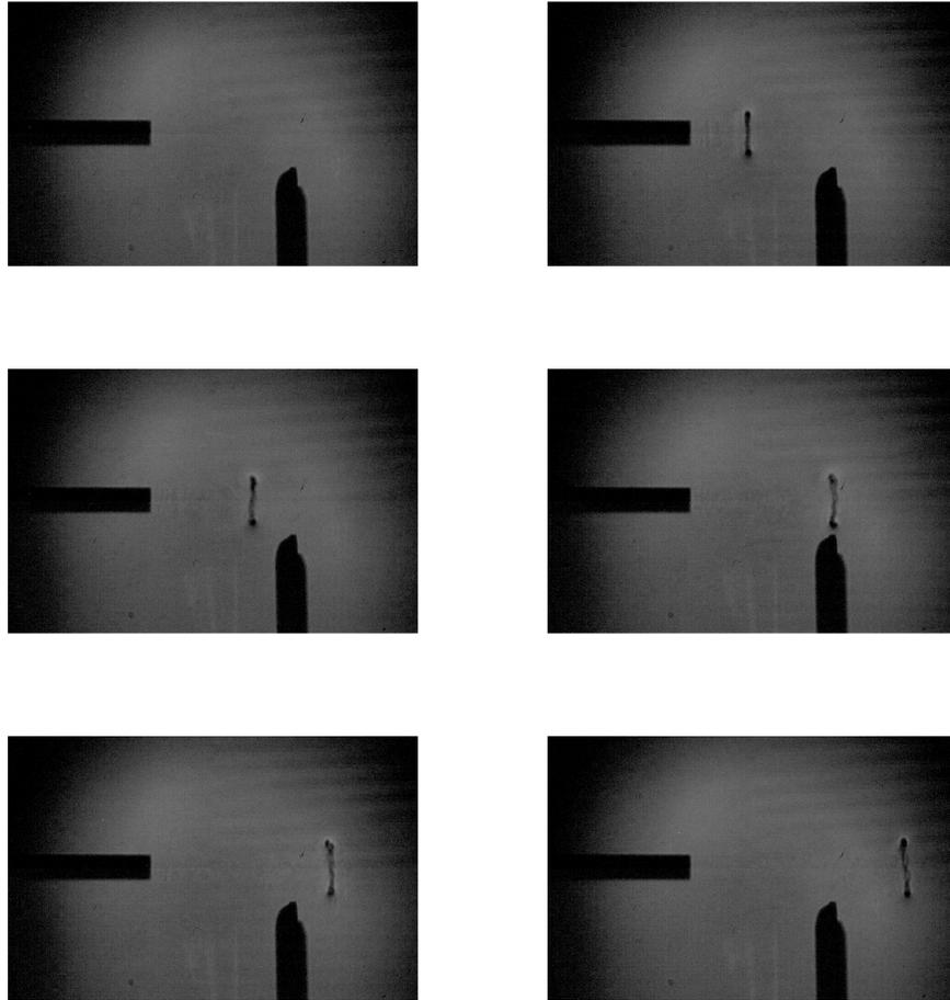
Figure 3.12: Schlieren high speed imaging of vortex ring formation and convection pathway near the plate when  $U_R = 62$  m/s,  $L = 9.8$ mm, and  $Z_p = 54$ mm.
