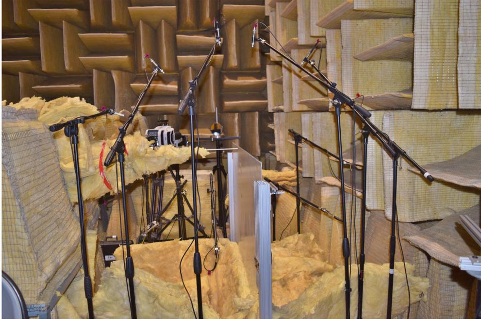
Figure 3.9: The 12 microphone array positioned central to the source region in the anechoic chamber.
