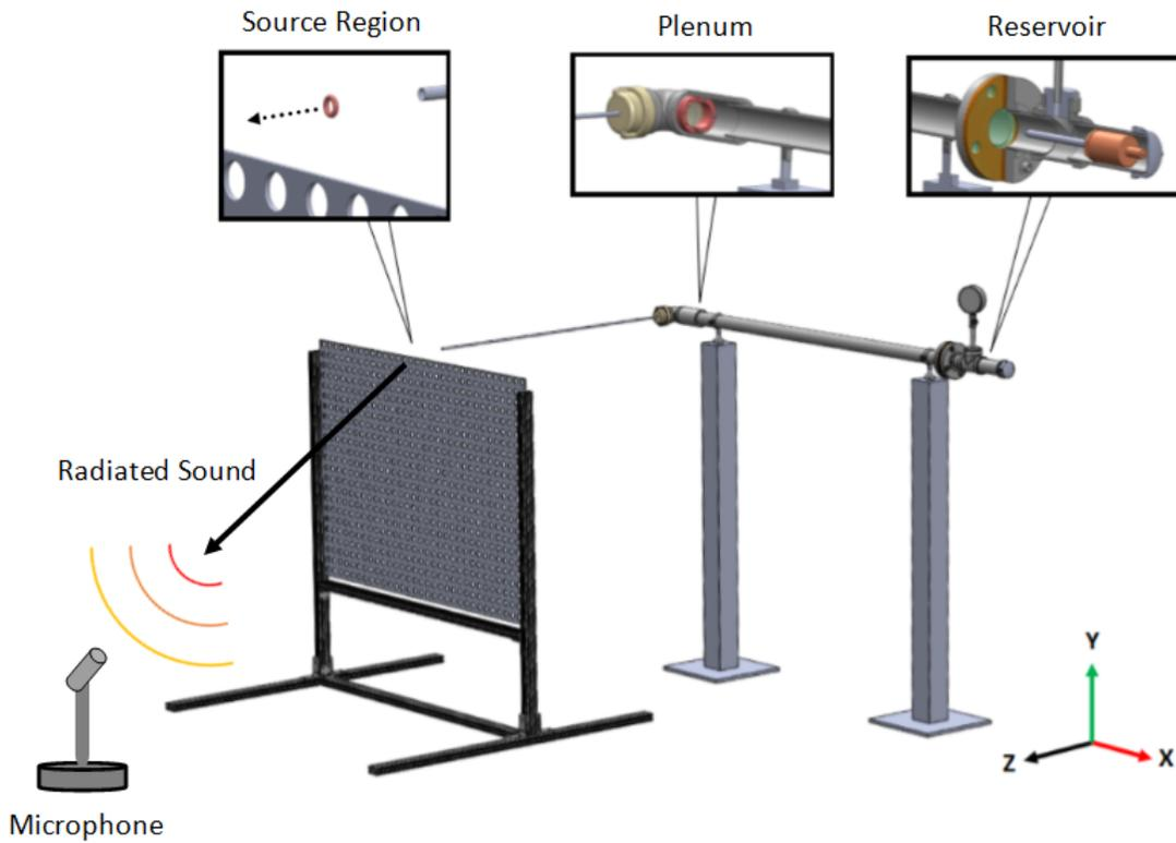
Figure 3.1: A schematic of the experimental setup, details shown for the vortex ring generator plenum, reservoir, source region, and microphones.
