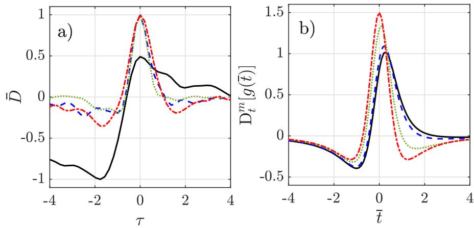
Figure 4.8: Comparison of experimentally computed  $\bar{D}$ , a), to predicted nondimensionalized source waveforms from Chen et al<sup>[1]</sup>, b). For a) -, -, :, and -. represent  $\mu/k = 0, 0.49, 3.10,$  and  $58.9,$  respectively. For b) -, -, :, and -. represent  $\mu/k \leq O(10^{-2}), 0.2, 1,$  and  $\geq O(10),$  respectively.
