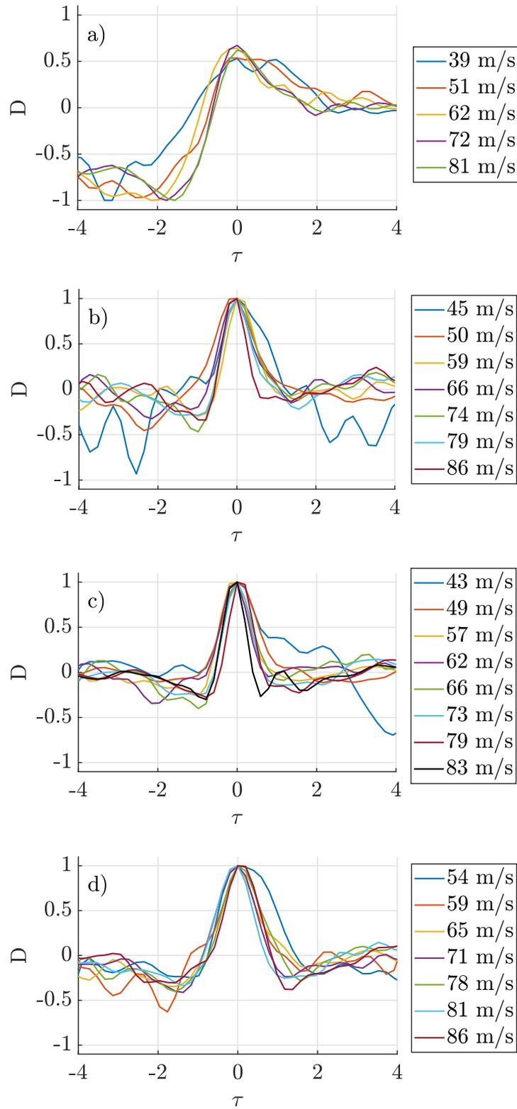
Figure 4.7: Nondimensionalized source waveforms,  $D$ , versus nondimensionalized time,  $\tau$  for (a)  $\mu/k = 0$ , (b)  $\mu/k = 0.49$ , (c)  $\mu/k = 3.10$ , and (d)  $\mu/k = 58.9$ . Line color and type indicate vortex ring speed shown in legends.
