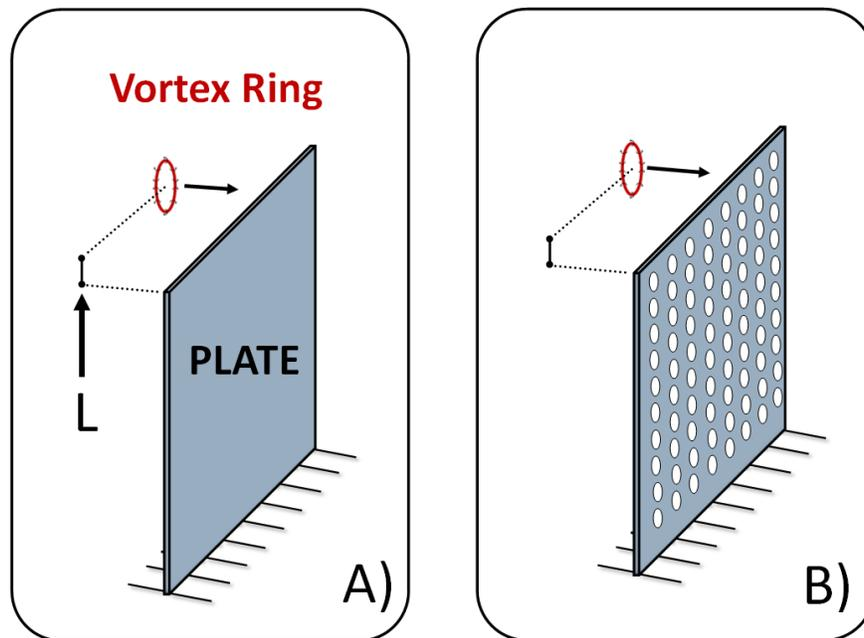
Figure 2.3: Schematic of a compact acoustic source, in the form of a vortex ring convecting near a) rigid impermeable plate and b) non-compact rigid porous plate.
