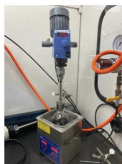
Step 6: Mechanically stir for one hour at 290rpm at 70C
