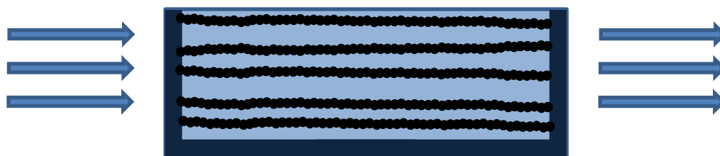
Figure 1-8: Chain formation of particles under the influence of an external magnetic field
