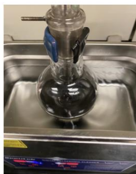
Step 4: Mechanically stir for one hour at 290rpm at 40C
