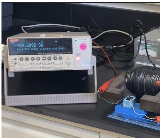
Figure 2-19: Resistance reading of the sample with a Keithley source meter, under a magnetic field applied using an electromagnet
