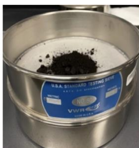
Step 1: Sieve iron oxide microparticles
