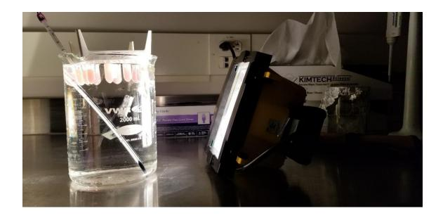
Figure 1: The photoactivation setup utilized for activation of the DNA intercalating agents. Clear 2 mL microcentrifuge tubes containing the samples and dyes were immersed in a 25°C water-filled beaker; water temperature was monitored and did not exceed 30°C during photoactivation. The halogen lamp was placed 20 cm away from the beaker and turned on for 15 minutes; the samples were rotated 180° at 7.5 minutes to allow for even distribution of light.
