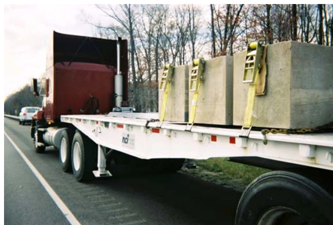
Figure 3.3: Truck with moveable weights for pavement loading
