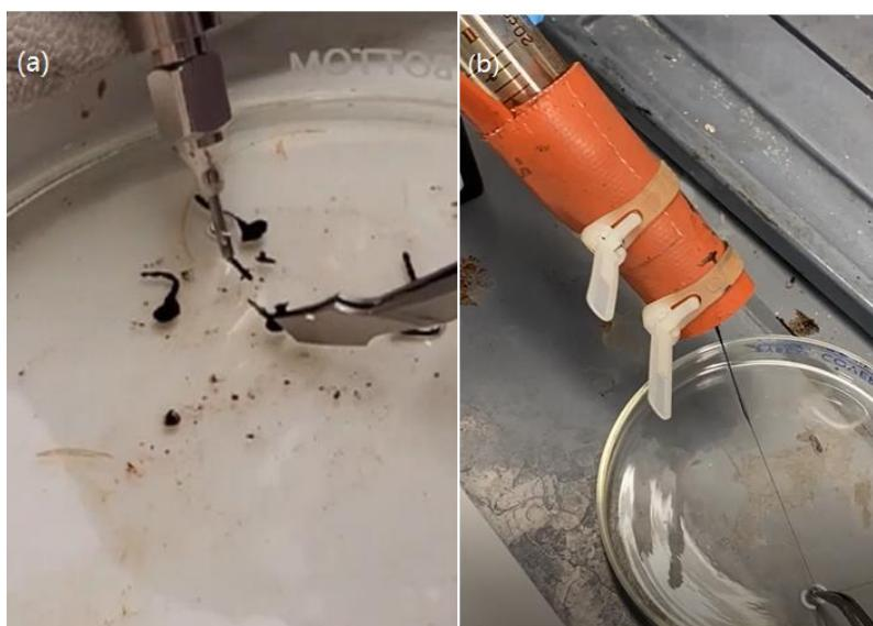
Figure 5.9 Pictures of PE-g-Pitch(8.4%)/TCB solutions showing (a) no spinnability and (b) good spinnability in the coagulation bath.
