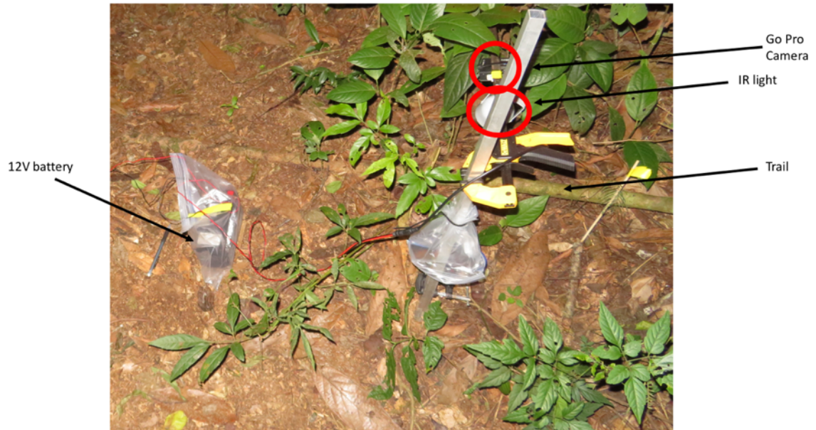
Figure AA-1. Image of field camera set-up for filming ants on trails.
