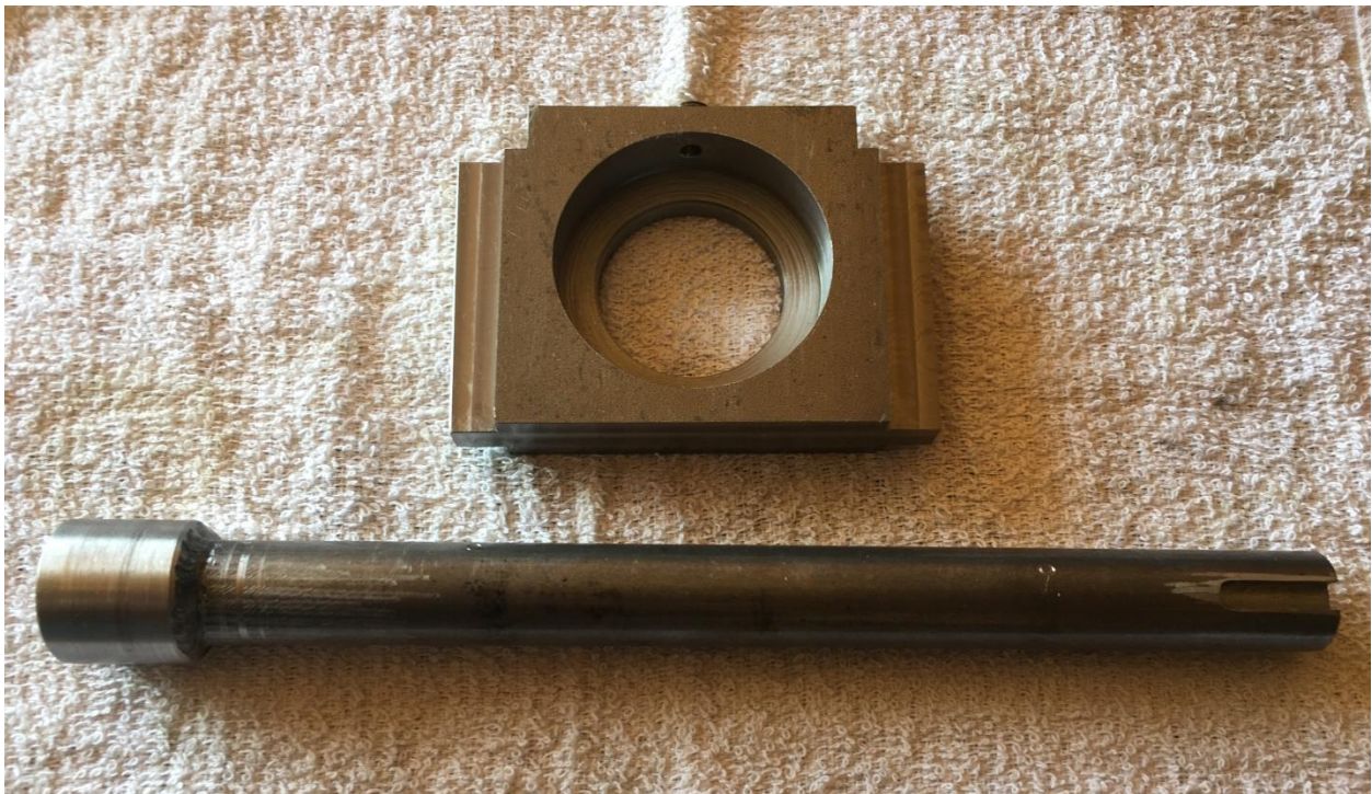
Figure 8: Bearing housing and shaft used for bearing with 72 mm OD bearings
