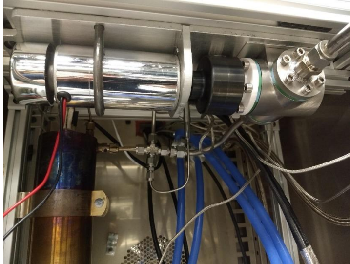
Figure 5-9: Turbine magnetically coupled with DC motor
