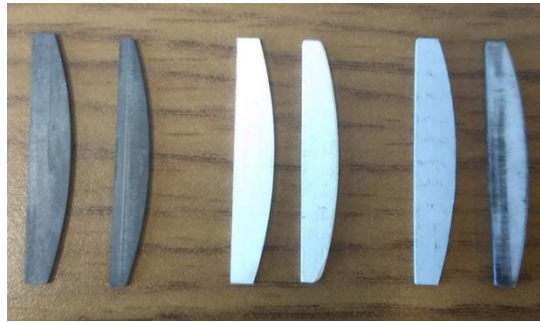
Figure 5-17: RVE vanes before and after testing. Graphite (left), hBN (middle), hBN-AlN (right)
