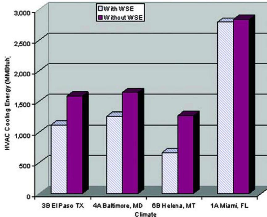
Figure 2-8: Waterside economizer energy savings in four climates (Stein, 2009)
