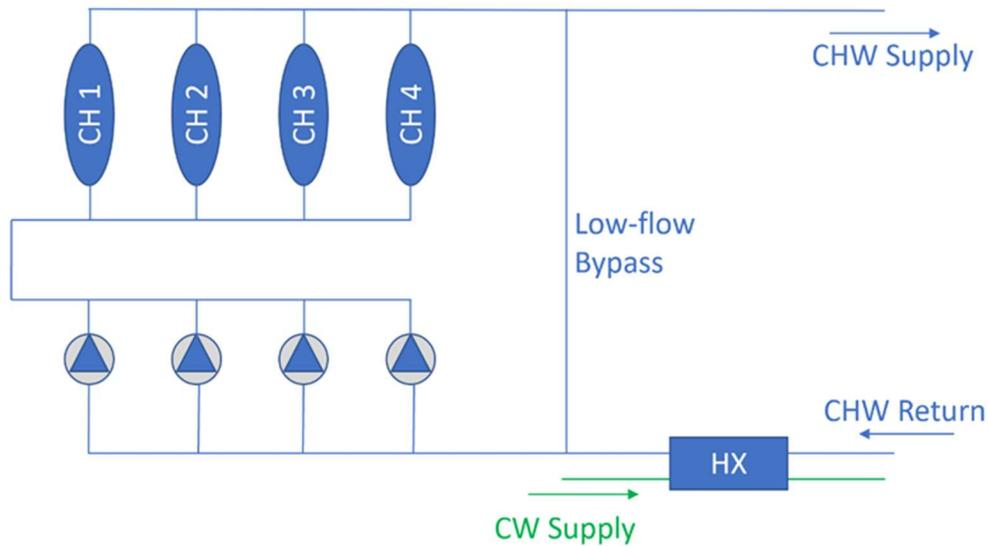
Figure 4-2: Chilled water system model flow diagram
