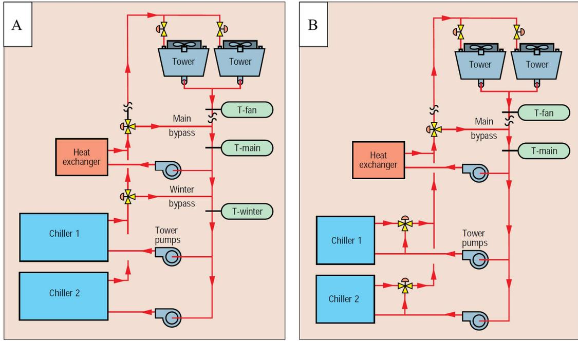
Figure 2-5: Chiller Control: A) Winter Bypass Control B) Heat Pressure Control (Kelly, 1996)
