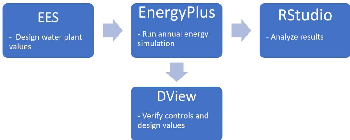
Figure 4-4: Parametric study computational flow chart
