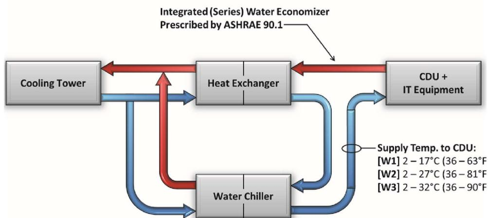
Figure 2-2: Liquid-cooled guidelines for data center classes (ASHRAE TC 9.9, 2015)
