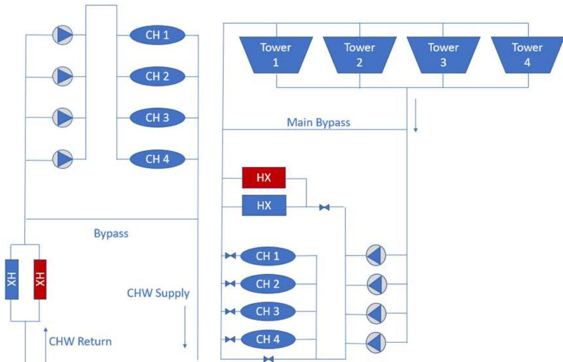
Figure 5-16: Alternative mission critical WSE design configuration
