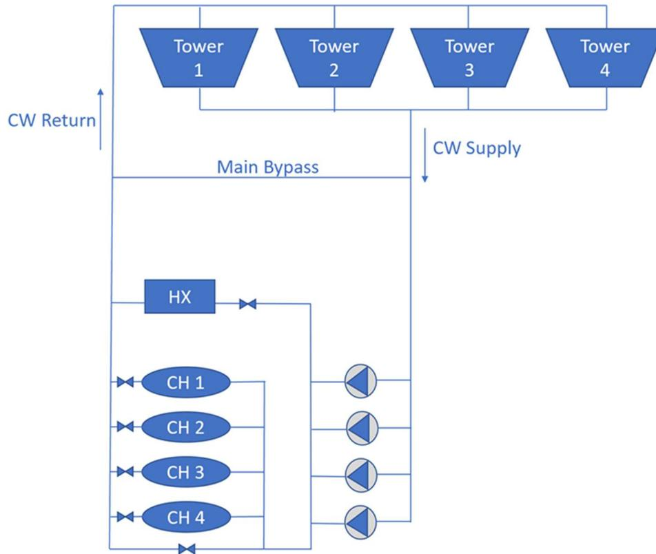
Figure 4-3: Condenser water system model flow diagram
