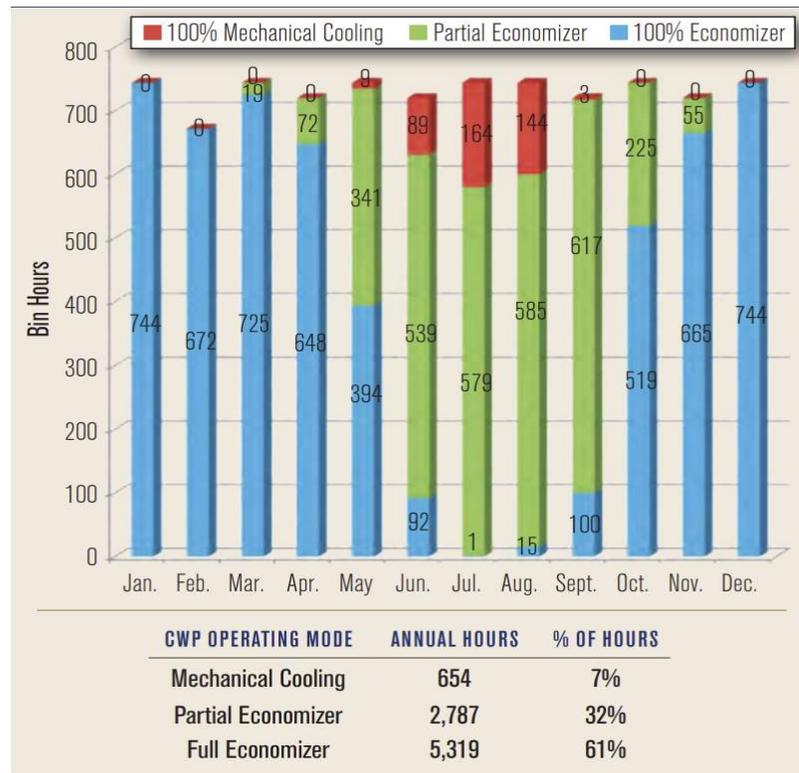
Figure 2-9: Bin hours for Chicago’s data center chiller plant operation (Griffin, 2015)
