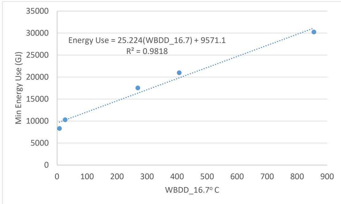
Figure 5-12: Minimum energy use vs WBDD
