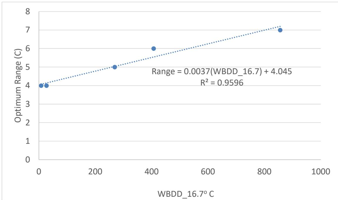
Figure 5-14: Optimum range vs WBDD
