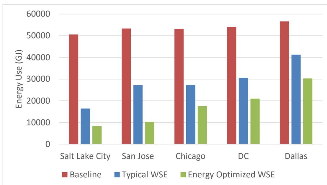
Figure 5-11: Energy savings of optimized waterside economizers
