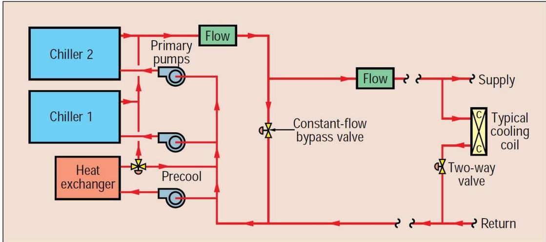
Figure 2-6: Preferred primary-only free cooling heat exchanger location (Kelly, 1996)
