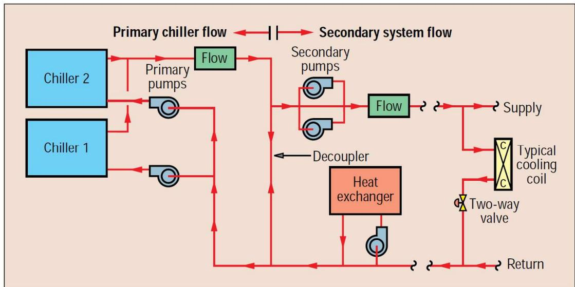
Figure 2-7: Preferred primary-secondary free cooling heat exchanger location (Kelly, 1996)
