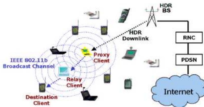
Figure A-1: 3G Cellular Network integrated with Wireless LAN Sensor Adhoc Network
