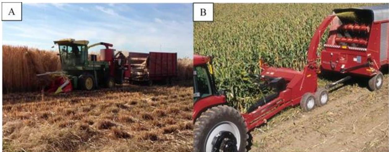
**Figure 2.5 – Self-propelled (A) and pull-behind forage chopper**
