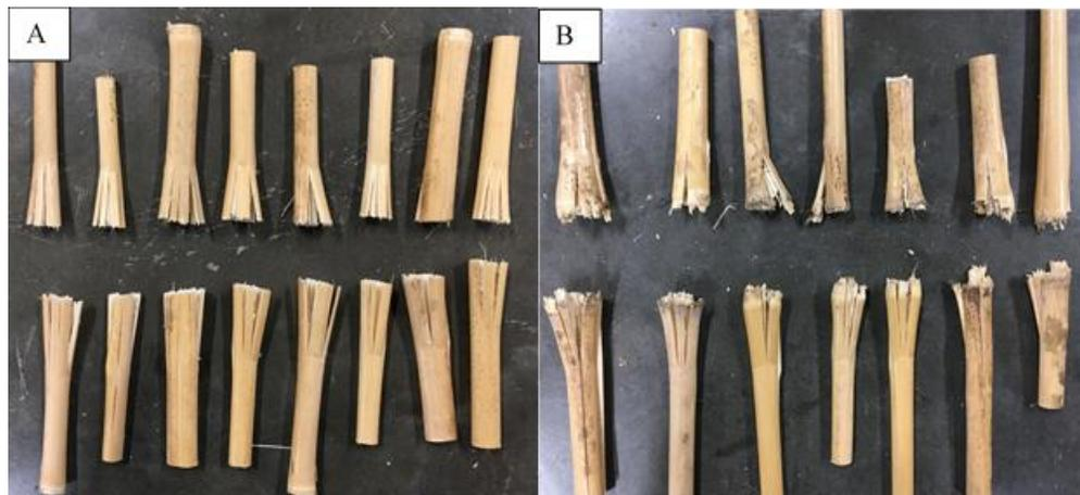
**Figure 5.14 – Illustration of cut sample using a serrated blade with both sides supported method. A- internode section, B – node section**
