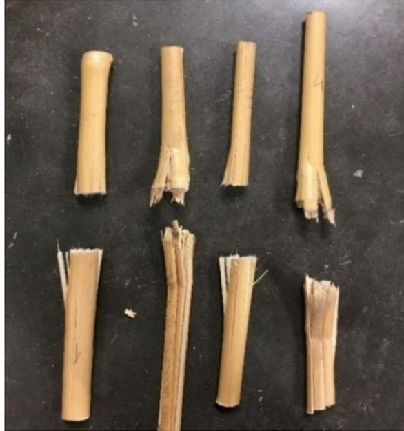
**Figure 5.10 – Illustration of cut sample using a serrated blade with one side supported method**
