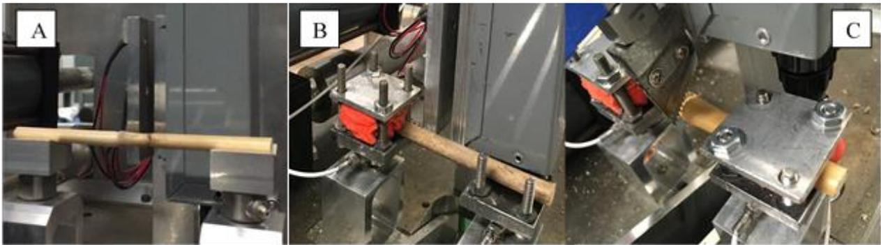
**Figure 4.12 – Unsupported cutting (A), one side supported cutting (B), two sides supported cutting (C)**
