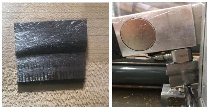
**Figure 4.9 – Fabricated flat blade used for the experiment**
