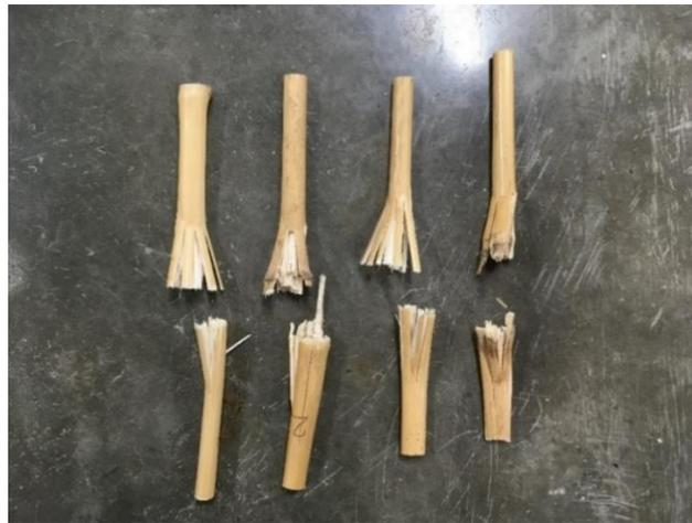
**Figure 5.1 – Illustration of cut sample using a flat blade with one side supported method**
