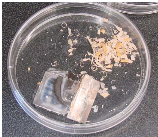
Figure 5.11: After \approx 24 hours of drying in air, the titania nanotube array membrane removed from the Ti foils samples in the foreground mechanically fracture into the shards seen in the upper right; the diameter of Petri dish is 90 mm.
