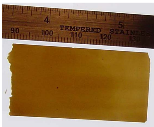
Figure 5.12: A completely stable, mechanically robust nanotube array membrane after critical point drying. The 200 \mu\text{m} thick membrane, 120 pore diameters, is approximately 2.5 cm x 4.5 cm.
