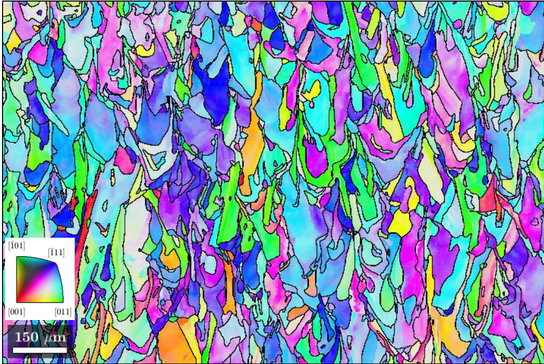
Figure 11. Results from the EBSD analysis of 316L. Build direction is upward on the page. The legend on the right communicates the relationship between grain orientation and color.
