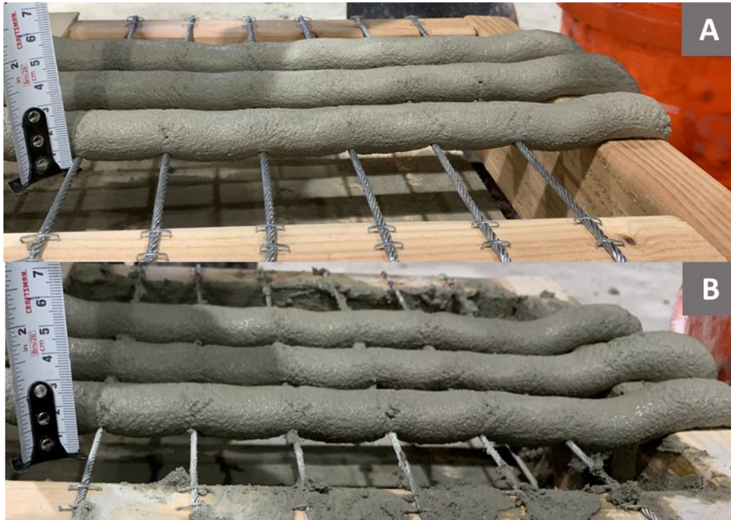
Figure 5-6: Wire cutting into concrete, 1/8-in wire in A and 3/32-in in B
