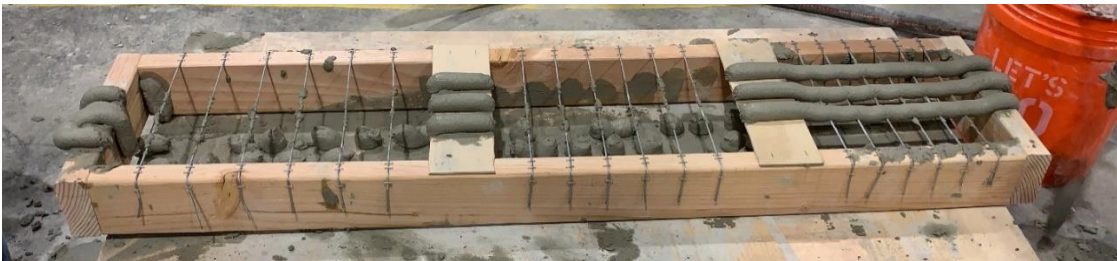
Figure 5-3: Bridging wire test
