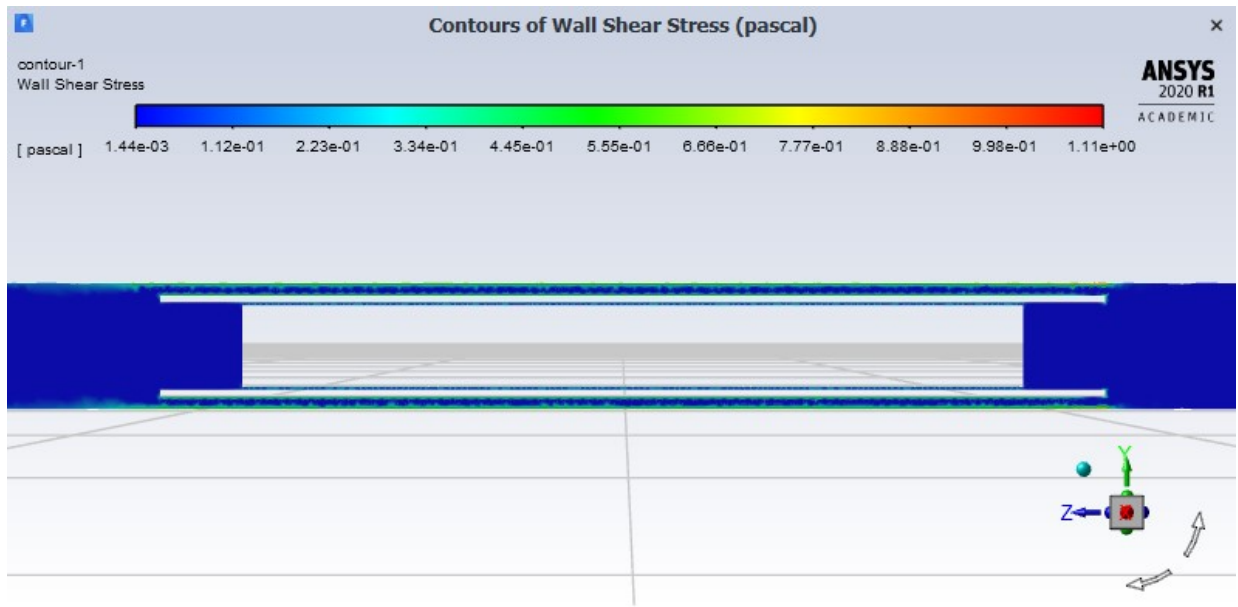
Figure 3.44: Wall shear stress of test section, 40 mm ID & 45 mm OD, 2e8 W/m 3 load
