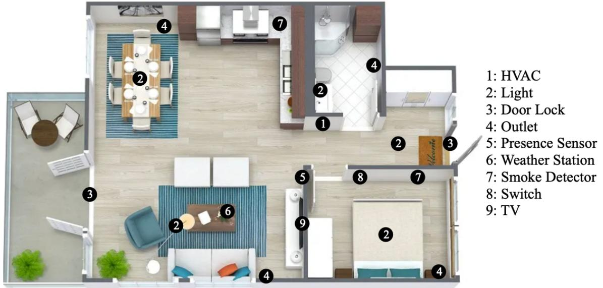
**Figure 4.1.** Floor plan of the experimental testbed
