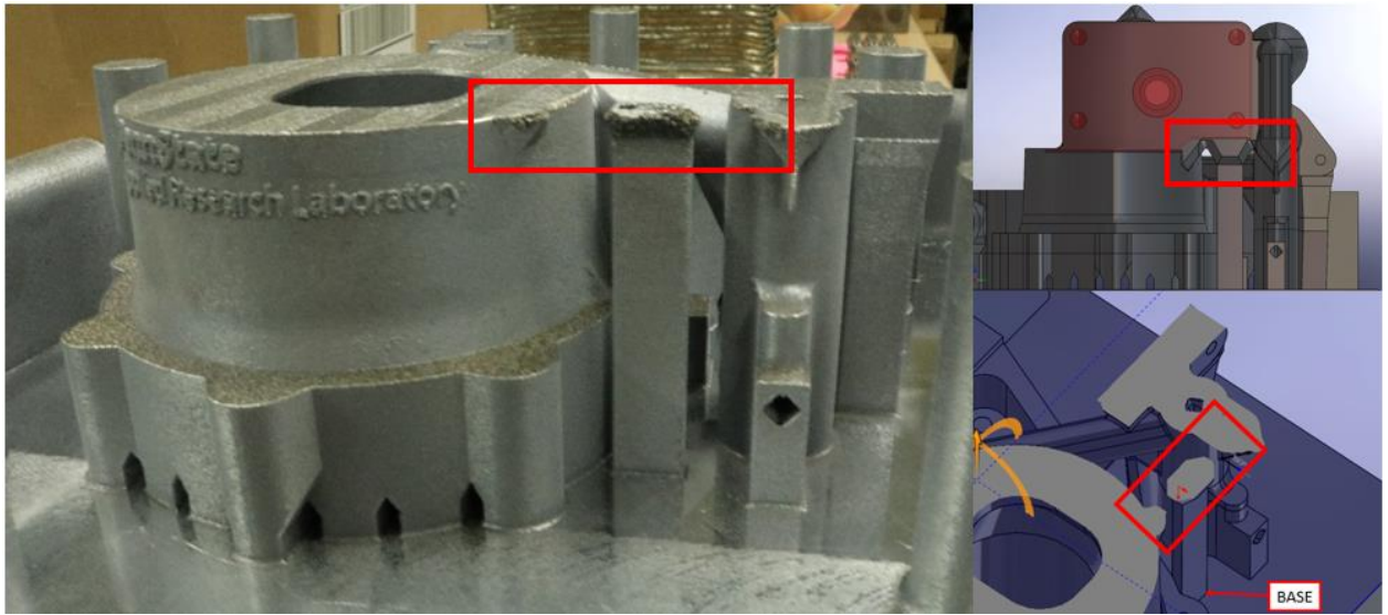
Figure 4-27: The build failure which necessitated a redesign of the support material. The base was 3 mm x 10 mm which flowered out at a 45 degree angle to anchor a large block of material several inches from the build plate.
