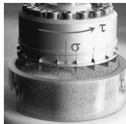
Fig. 5-2 Schematic diagram of the shear cell principle [36]
