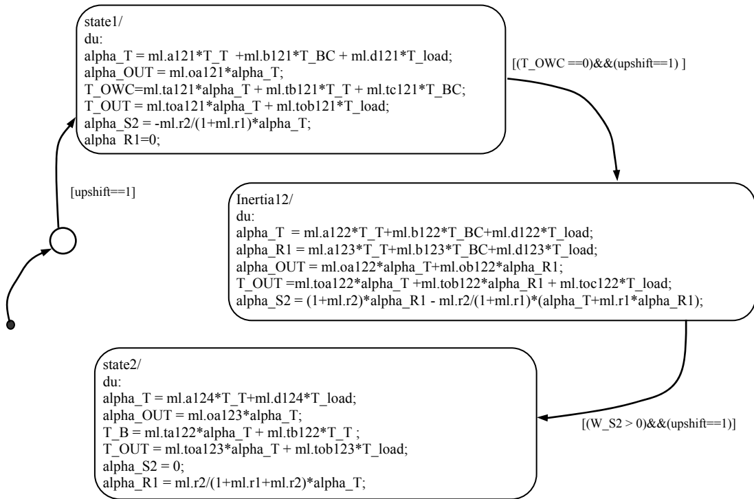
Figure 4-10: State chart for power on 1 \rightarrow 2 up shift simulation of A/T
