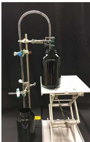
Figure 4-1. U-shape glass siphon utilized for removing the WAF from amber mixing jars.
