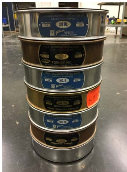
Figure 3-1. A stack of sieves with a cover on top and a pan for fines at the bottom
