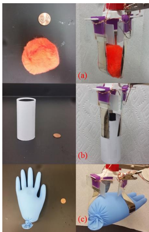
Figure 5-3. Grasping experiments for several target objects including (a) a 60 mm pom-pom ball, (b) a paper cylinder and (c) an inflated latex glove.
