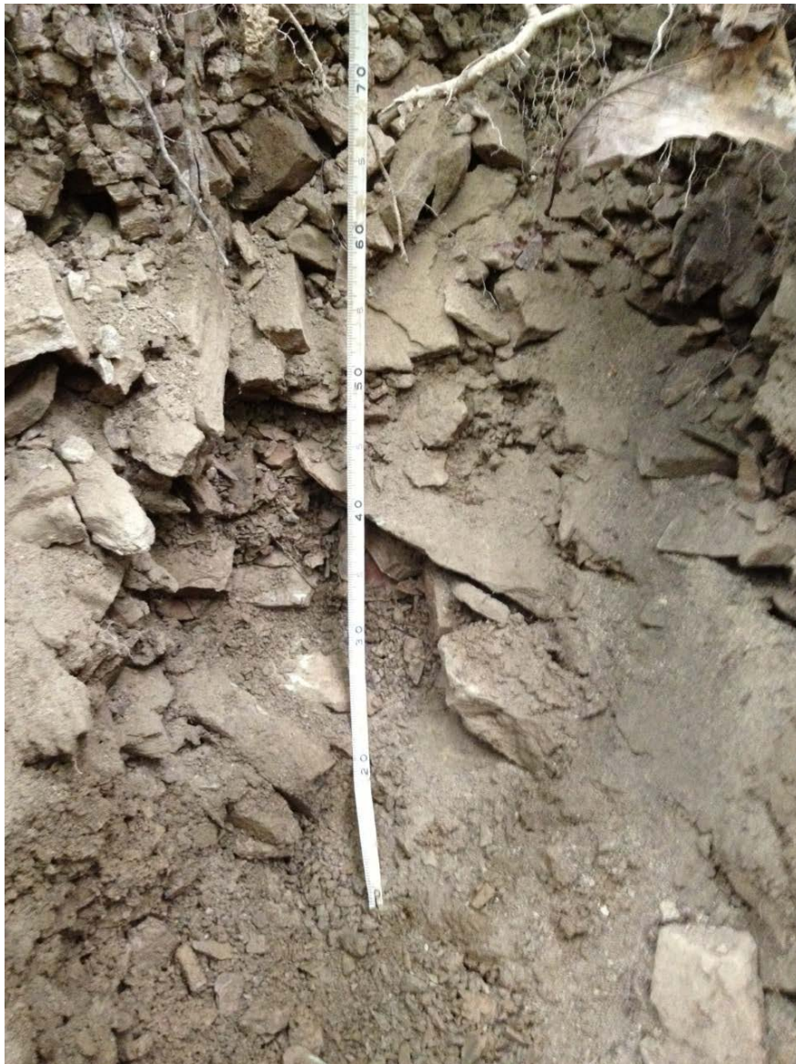
Photo B-1. SSHCZO site highly-fractured bedrock (photo credit: Andy Nyblade).
