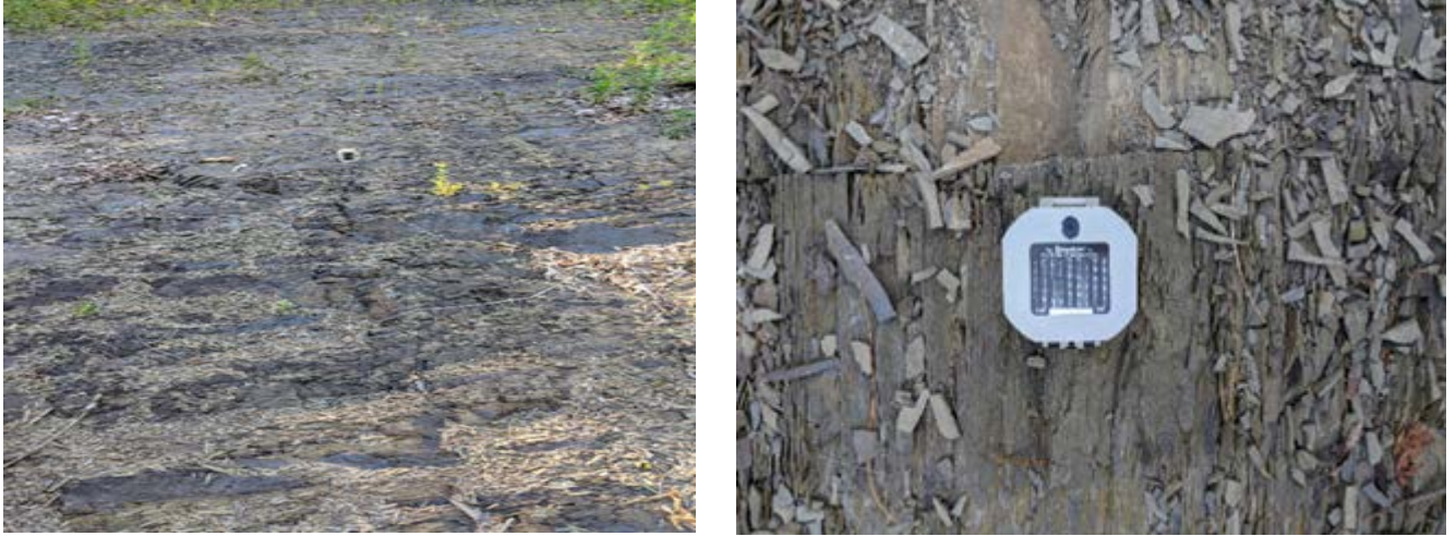
Figure 3-6. Shale outcrop near study area looking north along a joint (upper photo) with close up of shale (bottom photo) with a joint running left to right just above the compass and bedding running top to bottom along photo.
