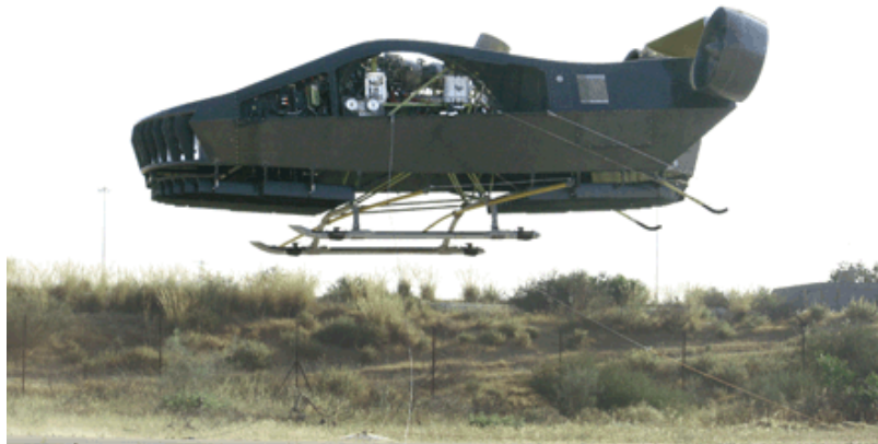
Figure 1-4 Urban Aeronautics AirMule in Hover Test (© Urban Aeronautics)
