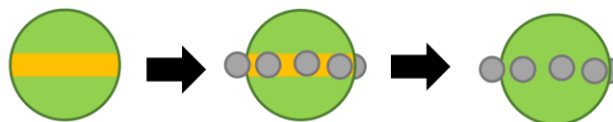
Figure 2: Schematic illustration of ring like deposition on a partially exchanged spherical particle
