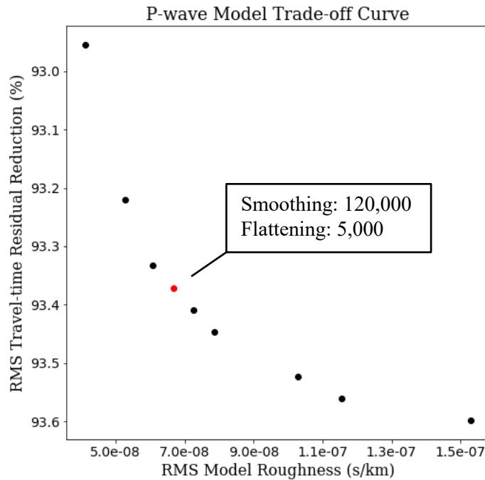
**Figure 2-6:** Trade-off curve for the P-wave model. Values plotted are from Table 2-1. The red point is the inversion parameters chosen for the final model, based on the trade-off curve.
