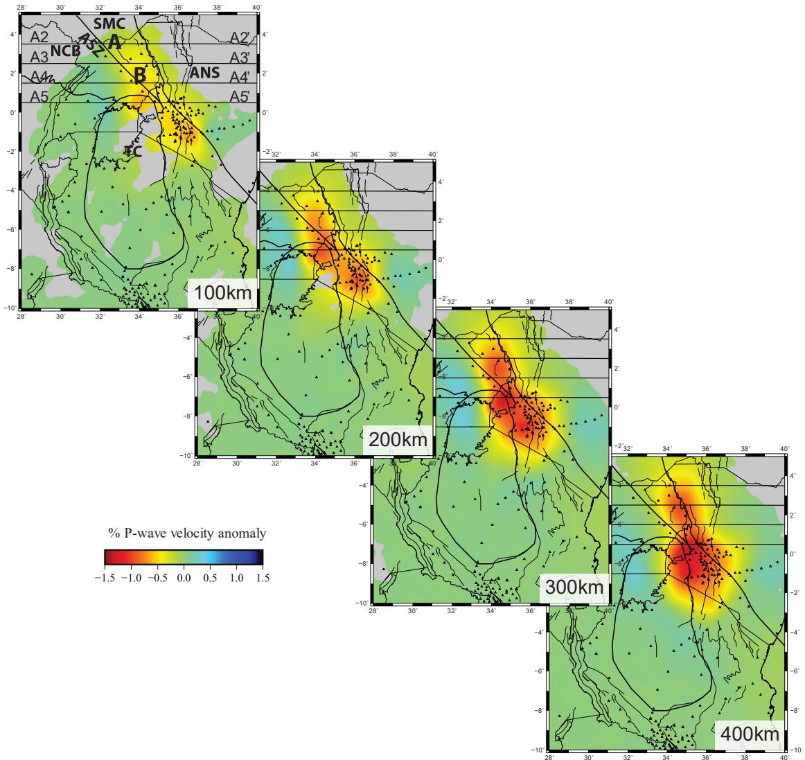
Figure 4-6: P-wave tabular body depth model sections at depths of 100, 200, 300, and 400 km. The position of vertical sections A2 to A5 are shown. Rifts and major geological boundaries are from *Katumwehe et al. [2016]* and Tanzania Craton boundary is from *Mulibo and Nyblade [2013]*. Triangles are stations used in the model. NCB – North Congo Block, SMC – Saharan Metacraton, ANS – Arabian-Nubian Shield, TC – Tanzania Craton, ASZ – Aswa Shear Zone.
