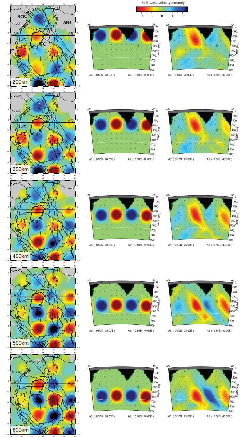
Figure 3-15: Comparison of S-wave checkerboard resolution results in map view (left), the input in cross section view (middle) and the output in cross section view (right) at depth intervals of 100 km from 100 km – 600 km. Geology from *Katumwehe et al. [2016]* and *Mulibo and Nyblade [2013]*. Triangles are stations used in the model. NCB – North Congo Block, SMC – Saharan Metacraton, ANS – Arabian-Nubian Shield, TC – Tanzania Craton, ASZ – Aswa Shear Zone.
