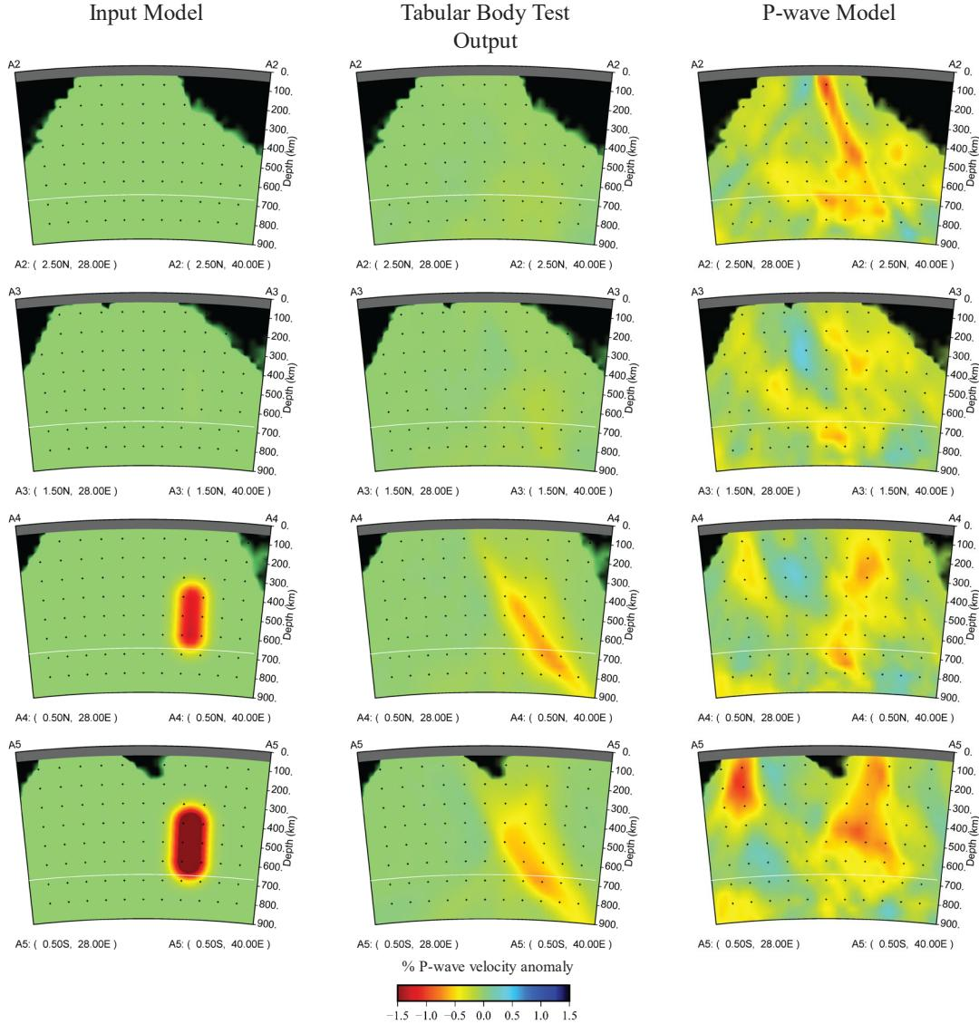
**Figure B-8:** P-wave Tabular body test input (left), Tabular body test results (center) and P-wave model (right) for A3-A3', A4-A4' and A5-A5' vertical cross sections from Figures 4-1, 4-2. And 4-3. The input model includes a 150 km long (N-S), 150 km wide (E-W), and 250 low wave-speed anomaly from depths of 400 to 600 km representing the previously imaged LWA underneath the Kenya Rift.
