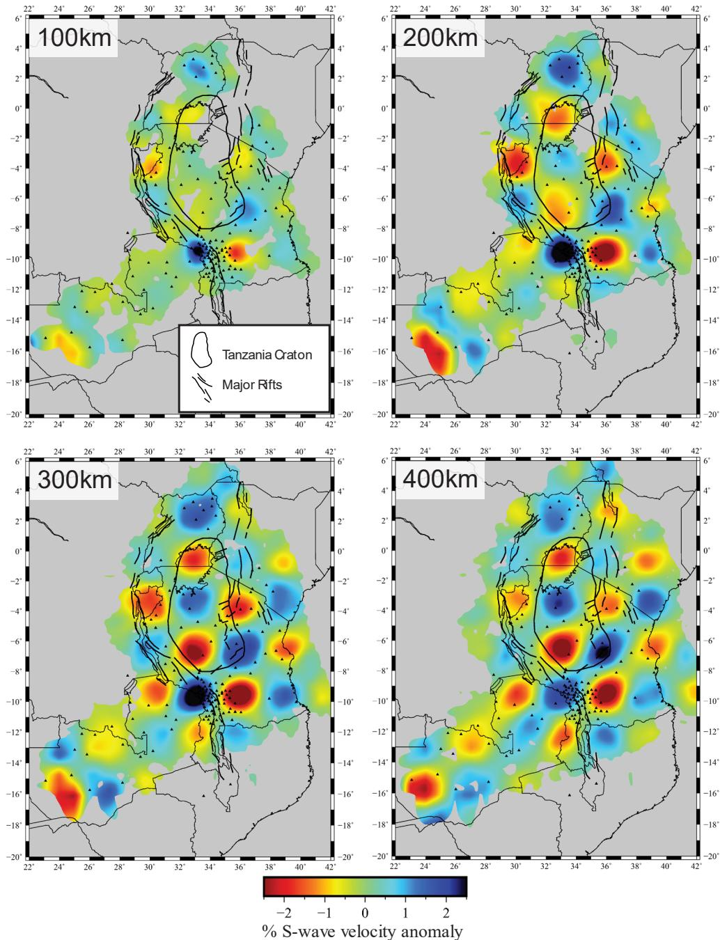
Figure 3-13: Depth sections of the 200 km wide S-wave checkerboard test results at 100, 200, 300, and 400 km depths. Geology from *Mulibo and Nyblade [2013]*. Triangles are stations used in the model.
