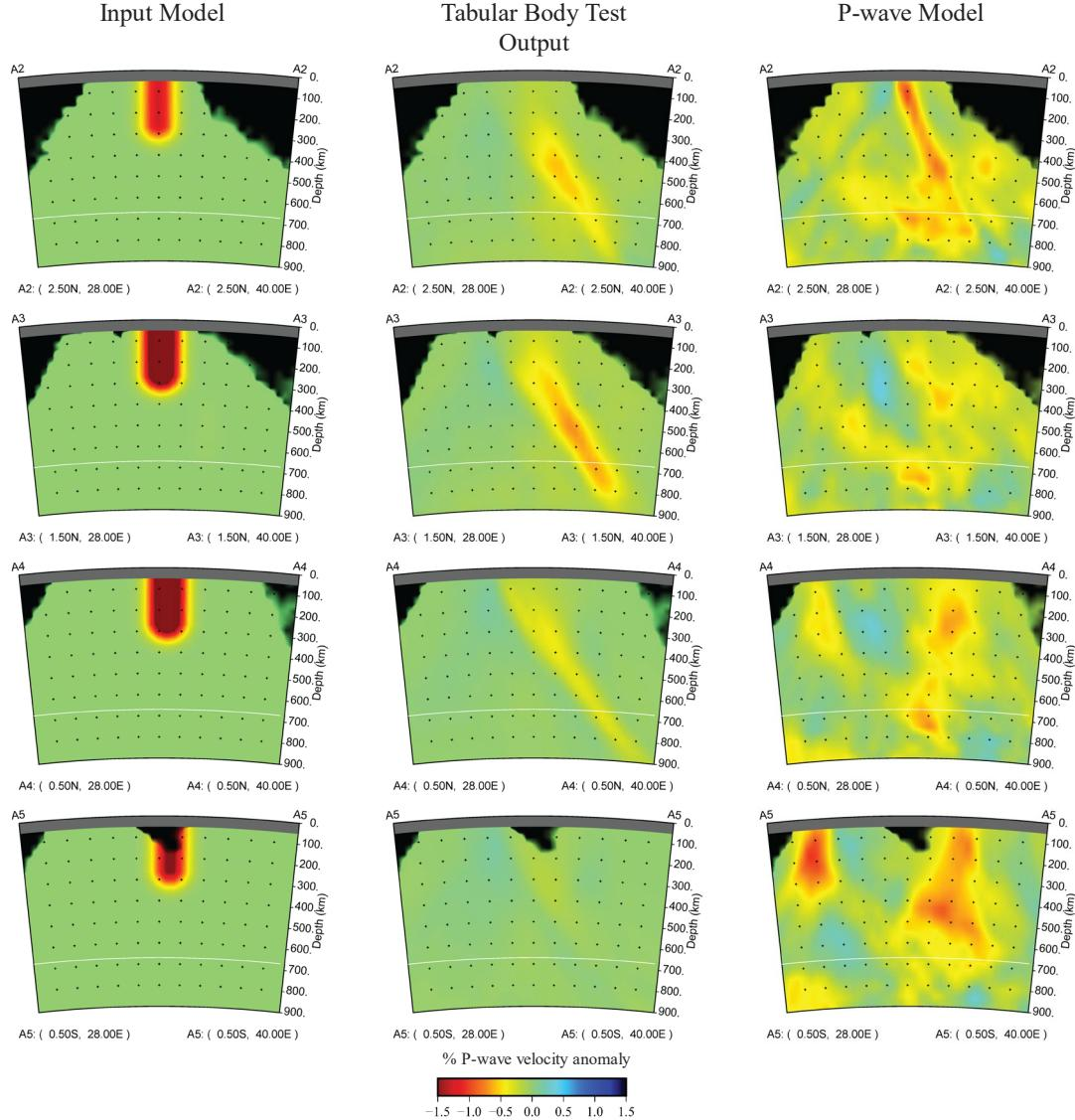
**Figure B-7:** P-wave Tabular body test input (left), Tabular body test results (center) and P-wave model (right) for A3-A3', A4-A4' and A5-A5' vertical cross sections from Figures 4-1, 4-2. And 4-3. The input model includes a 222 km long (N-S), 150 km wide (E-W), and 250 km deep low wave-speed anomaly representing Anomaly B.
