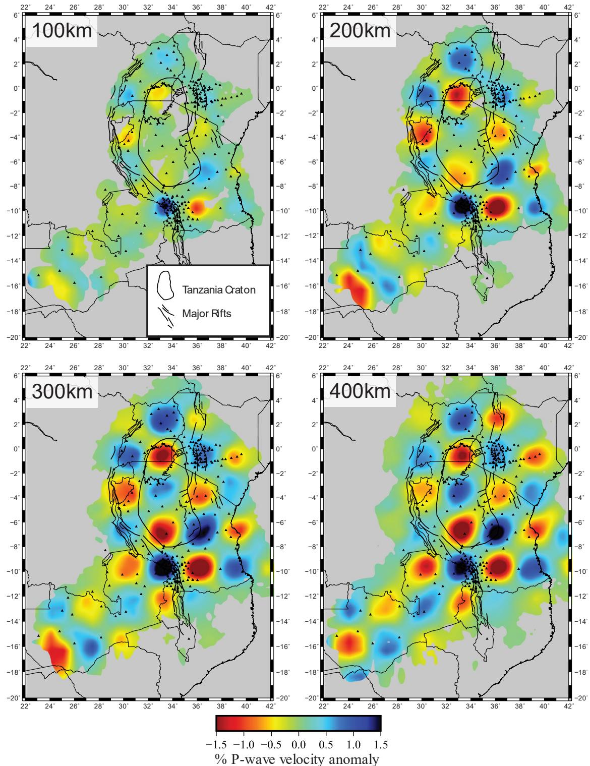
Figure 3-8: Depth sections of the 200 km wide P-wave checkerboard test results at 100, 200, 300, and 400 km depths. Geology from *Mulibo and Nyblade [2013]*. Triangles are stations used in the model.
