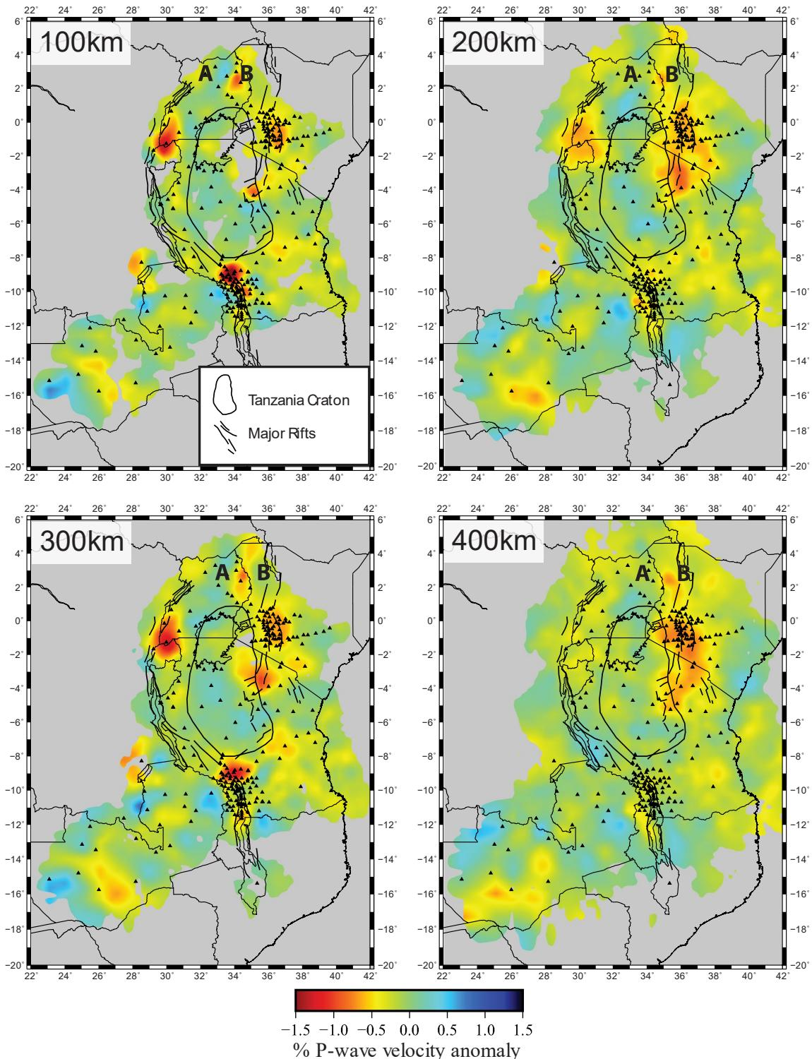
Figure 3-5: Horizontal sections through the P-wave tomography model at 100 km to 400 km depths. Geological features are from *Mulibo and Nyblade [2013]*. Triangles are stations used in the model.
