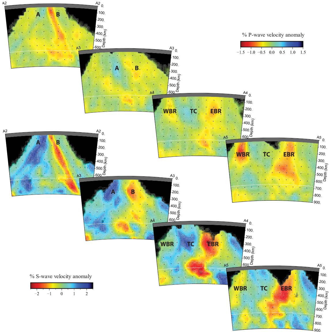
**Figure 4-4:** Vertical sections A2 to A5 from the P-wave (top) and S-wave (bottom) body-wave tomography model. Location of the sections are shown in Figure 4-1 and 4-2. A – Anomaly A FWA, B – Anomaly B LWA, WBR – Western Branch, TC – Tanzania Craton, EBR – Eastern Branch.
