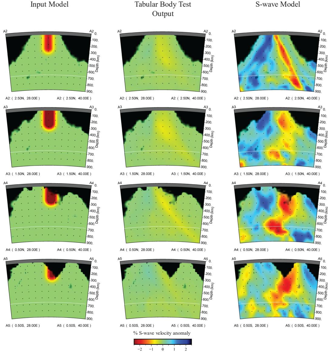
**Figure B-9:** S-wave Tabular body test input (left), Tabular body test results (center) and P-wave model (right) for A3-A3', A4-A4' and A5-A5' vertical cross sections from Figures 4-1, 4-2. And 4-3. The input model includes a 222 km long (N-S), 150 km wide (E-W), and 250 km deep low wave-speed anomaly representing Anomaly B.
