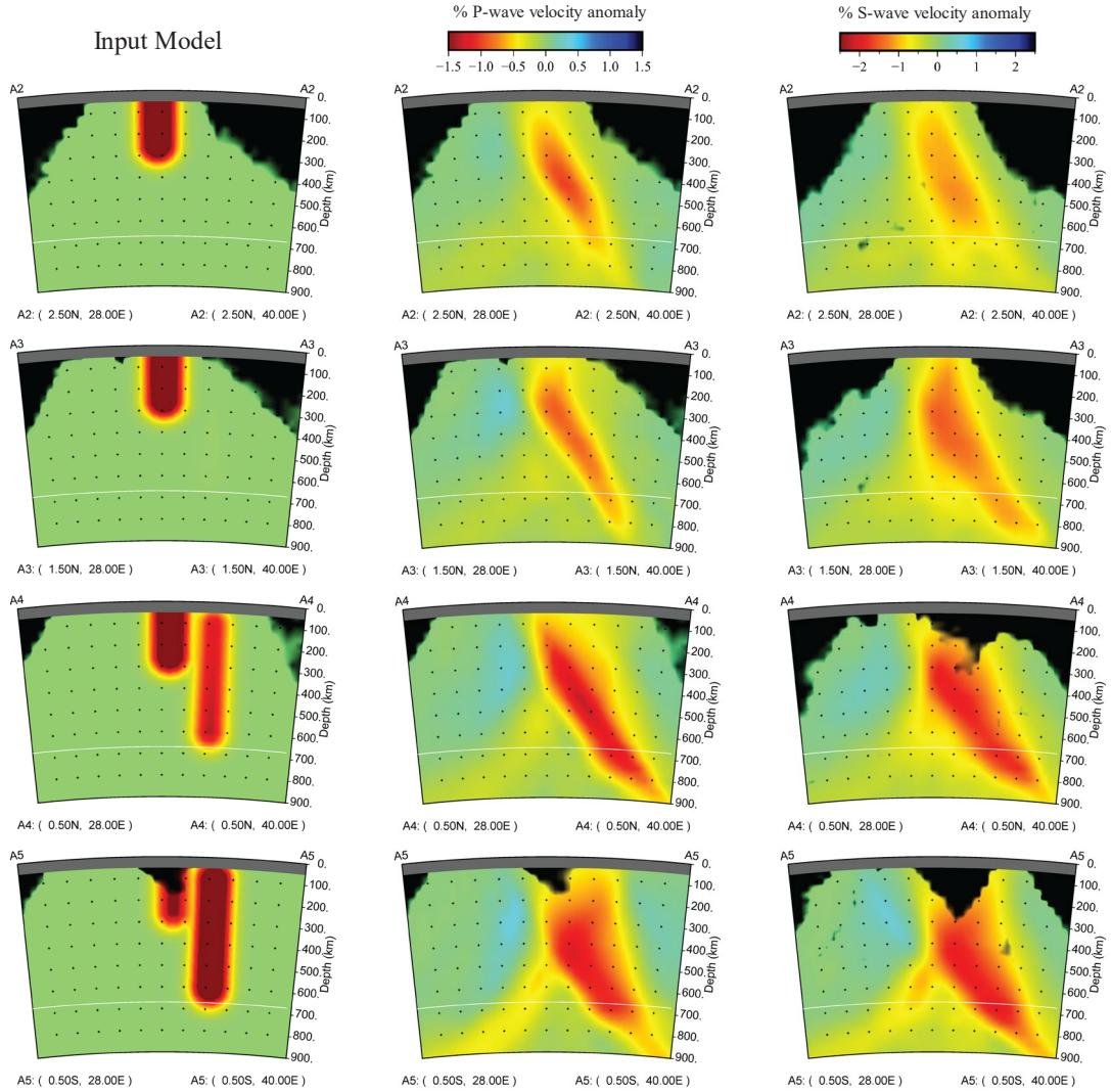
Figure 4-8: Tabular body test input (left), P-wave model results (center) and S-wave model results (right) for A3-A3', A4-A4' and A5-A5' vertical cross sections from Figures 4-1, 4-2. And 4-3. The input model has tabular bodies for both Feature B and the LWA from preview models.
