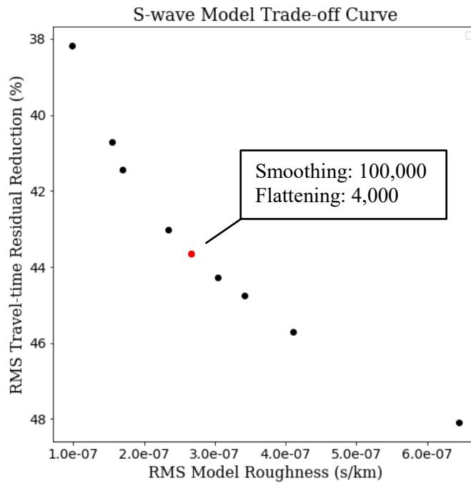
**Figure 2-9:** Trade-off curve for the S-wave model reduction due to the effects of station terms, source terms and earthquake relocations. Values plotted are from Table 2-4. The red point is the inversion parameters chosen for the final model, based on the trade-off curve.
