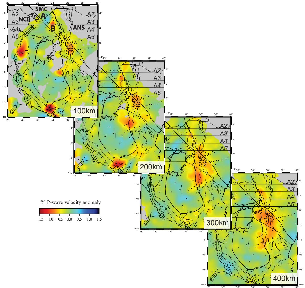
Figure 4-2: P-wave model depth sections at 100, 200, 300, and 400 km depths. Rifts and major geological boundaries are from *Katumwehe et al.* [2016] and Tanzania Craton boundary is from *Mulibio and Nyblade* [2013]. Triangles are stations used in the model. NCB – North Congo Block, SMC – Saharan Metacraton, ANS – Arabian-Nubian Shield, TC – Tanzania Craton, ASZ – Aswa Shear Zone.
