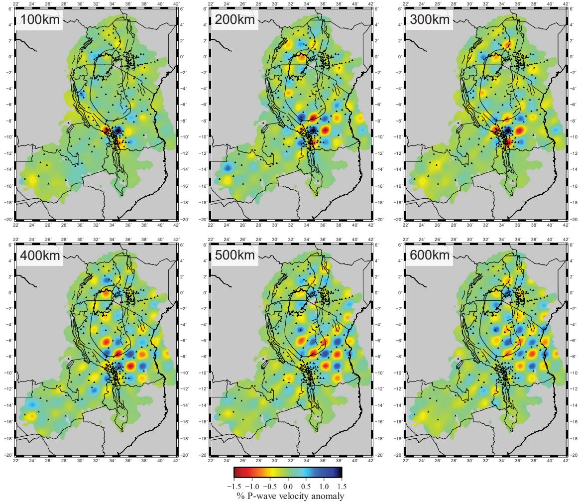
**Figure B-3:** Depth sections of the 100 km wide P-wave checkerboard test results at 100 km intervals from depths of 100 km to 600 km . Geology from [Mulibo and Nyblade, 2013].
