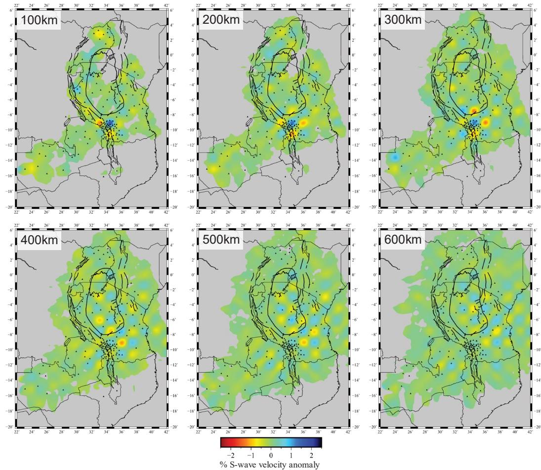
**Figure B-6:** Depth sections of the 100 km wide S-wave checkerboard test results at 100 km intervals from depths of 100 km to 600 km. Geology from [Mulibio and Nyblade, 2013].
