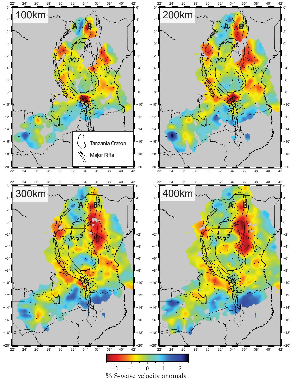
Figure 3-11: Horizontal sections through the S-wave tomography model at 100 km to 400 km depths. Geological features are from *Mulibbo and Nyblade [2013]*. Triangles are stations used in the model.
