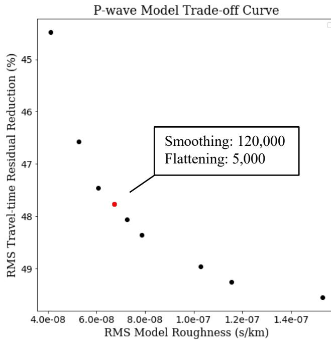
**Figure 2-8:** Trade-off curve for the P-wave model reduction due to the effects of station terms, source terms and earthquake relocations. Values plotted are from Table 2-3. The red point is the inversion parameters chosen for the final model, based on the trade-off curve.
