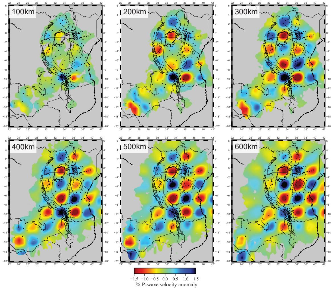
**Figure B-2:** Depth sections of the 200 km wide P-wave checkerboard test results at 100 km intervals from depths of 100 km to 600 km . Geology from [Mulibo and Nyblade, 2013].
