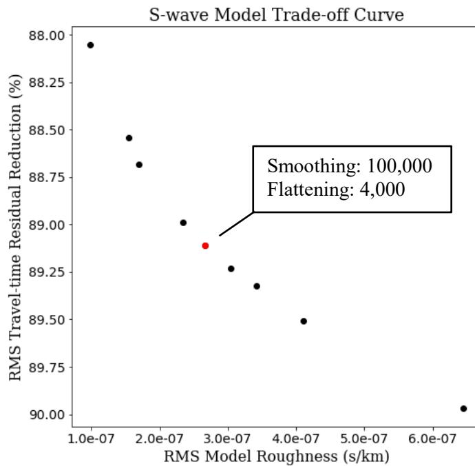
**Figure 2-7:** Trade-off curve for the S-wave model. Values plotted are from Table 2-2. The red point is the inversion parameters chosen for the final model, based on the trade-off curve.
