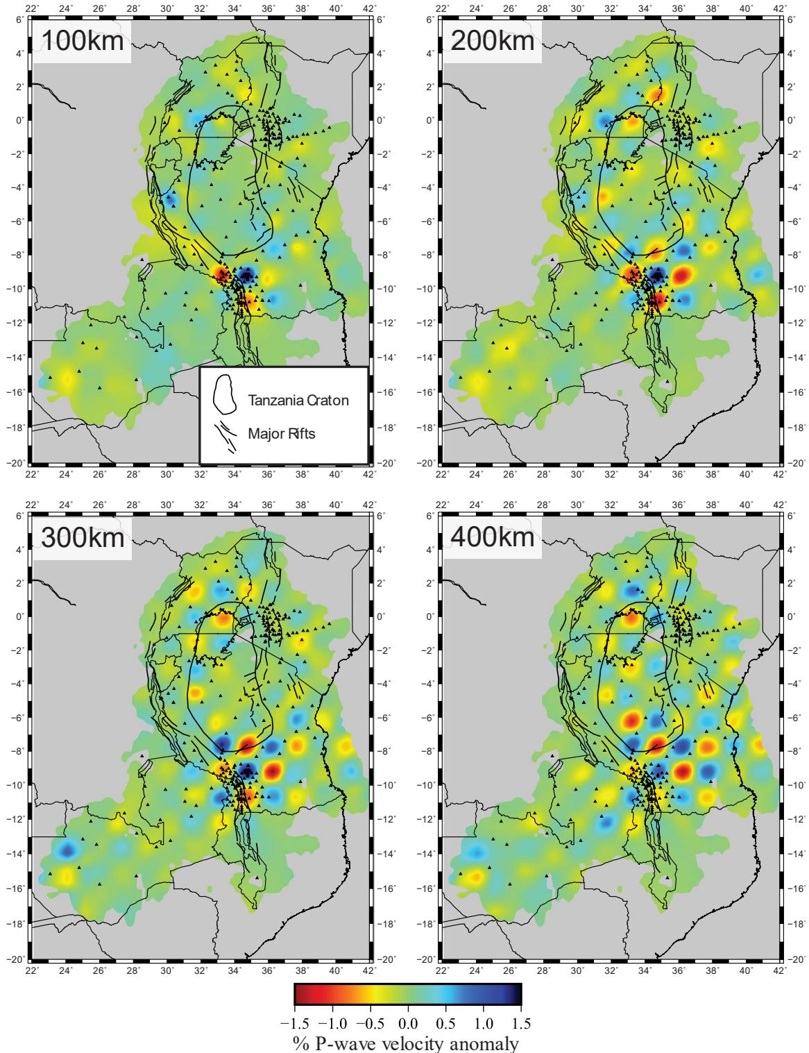
Figure 3-9: Depth sections of the 200 km wide P-wave checkerboard test results at 100, 200, 300, and 400 km depths. Geology from *Mulibo and Nyblade [2013]*. Triangles are stations used in the model.
