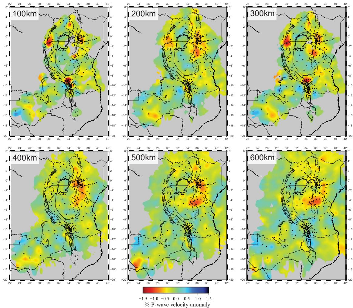
Figure B-1: Depth sections for the P-wave tomography model at depths from 100 km to 600 km at 100 km intervals. Geology from [Mulibo and Nyblade, 2013].
