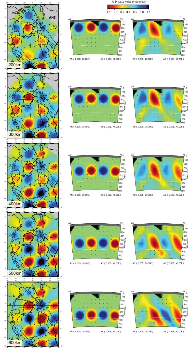
**Figure 3-10:** Comparison of P-wave checkerboard resolution results in map view (left), the input model in cross section view (middle) and the output in cross section view (right) at depth intervals of 100 km from depths of 100 km to 600 km. Geology from *Katumwehe et al. [2016]* and *Mulibo and Nyblade [2013]*. Triangles are stations used in the model. NCB – North Congo Block, SMC – Saharan Metacraton, ANS – Arabian-Nubian Shield, TC – Tanzania Craton, ASZ – Aswa Shear Zone.
