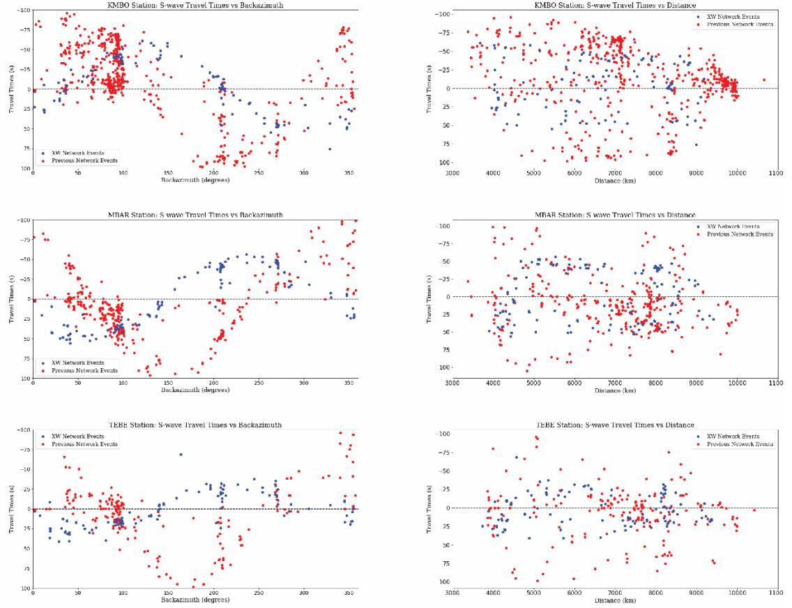
**Figure B-12:** S-wave travel-time residuals for collocated KMBO, TEBE, and MBAR stations vs back azimuth (left) and vs depth (right). The travel time residuals are derived from Section 2.3, Equation 2.3 where the preliminary expected travel time (based on the the IASPI91 velocity model) and the mean of expected travel times for the event are subtracted from the arrival time for the station.
