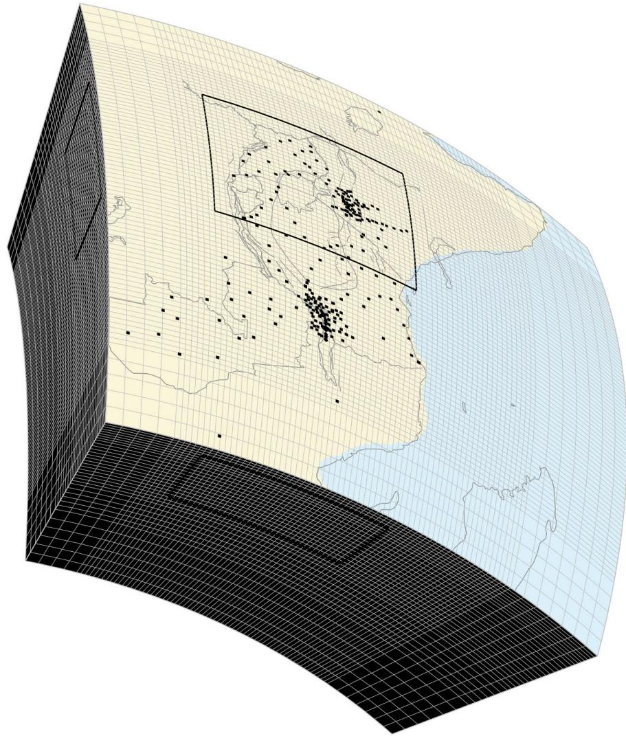
Figure 2-5: Visual representation of the model parameterization used in this study. Knots are densely spaced in the main study area, and less densely spaced towards the edge of the model. The black box represents the focus area of this study.
