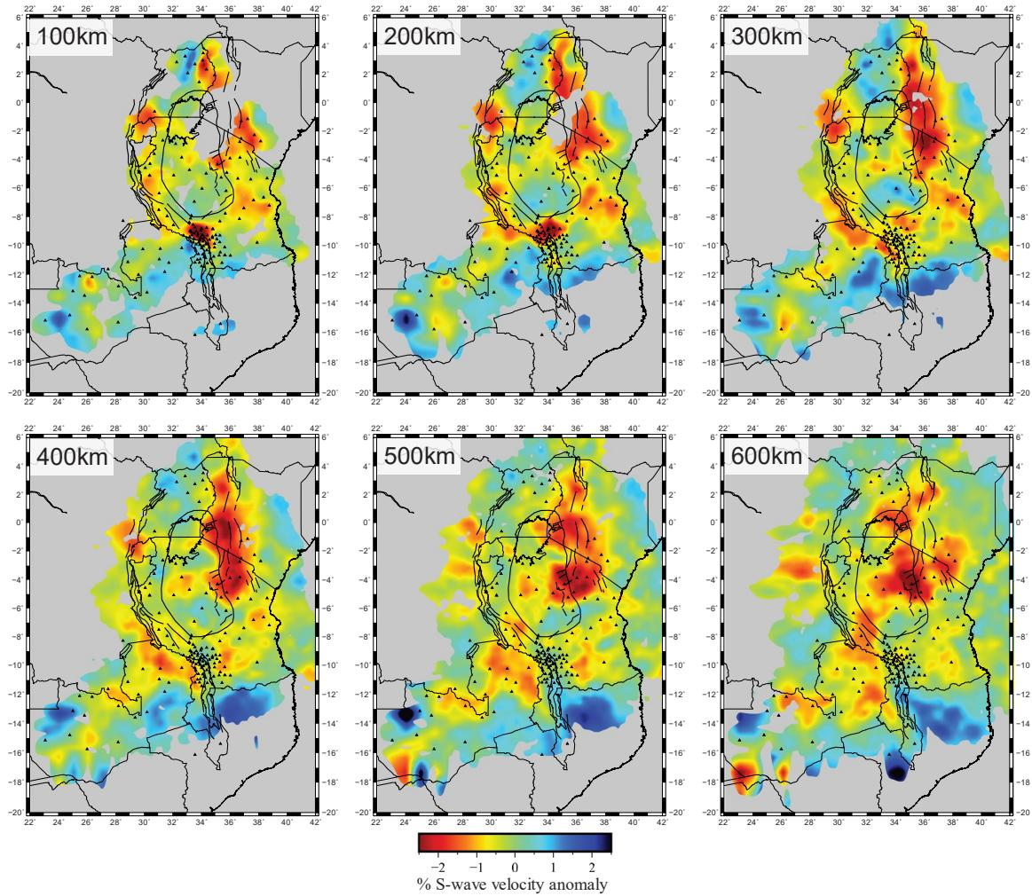
**Figure B-4:** Depth sections for the S-wave tomography model at depths from 100 km to 600 km at 100 km intervals. Geology from [Mulibo and Nyblade, 2013].
