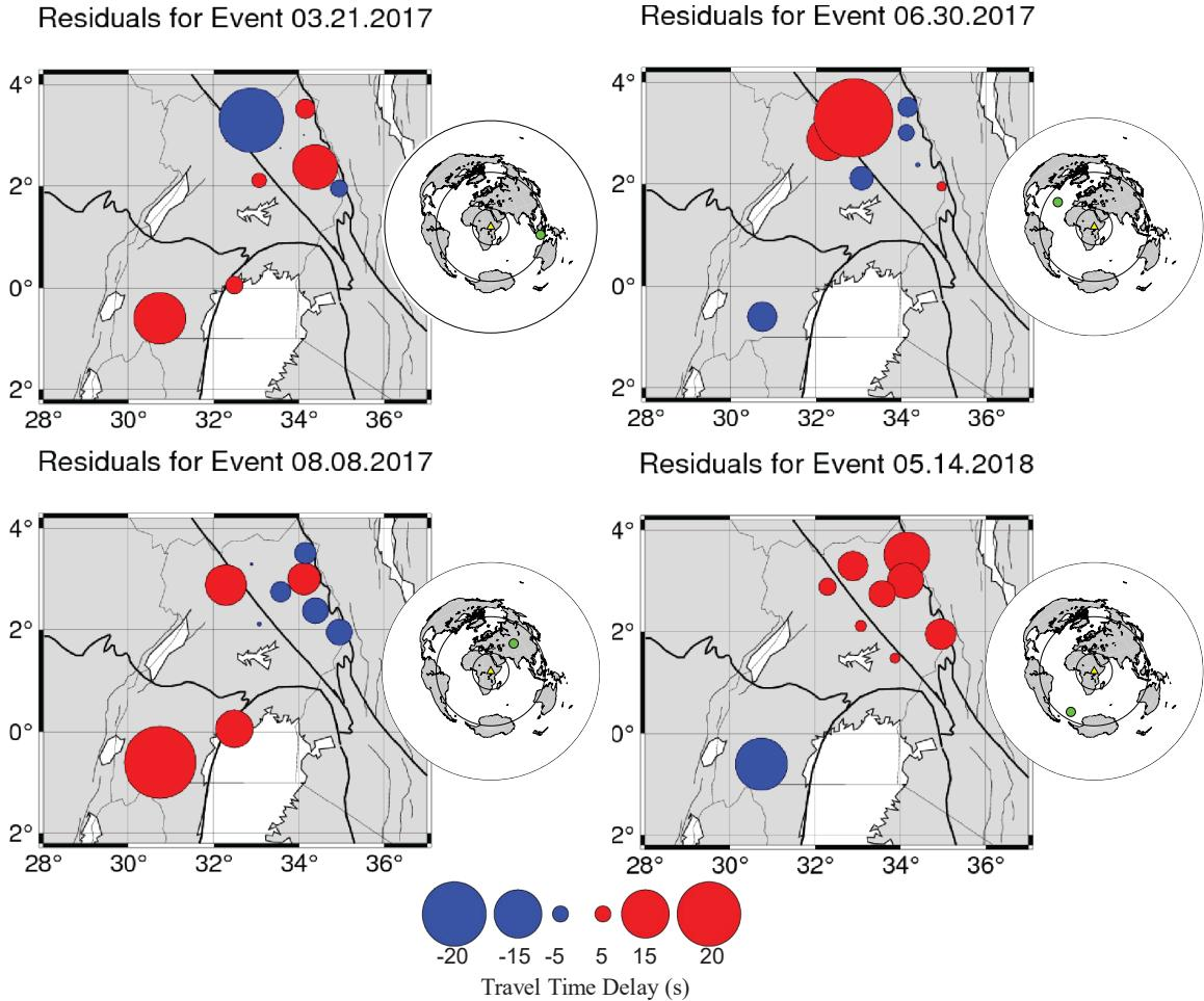
**Figure 3-1:** P-wave delay times for four events from 2017-2018. Inset map shows the location of the event (green dot). Circles are shown at distances of 30° and 90° away from the center of the network to indicate the range of teleseismic events. Geology is from *Katumwehe et al. [2016]* and *Mulibø and Nyblade [2013]*.
