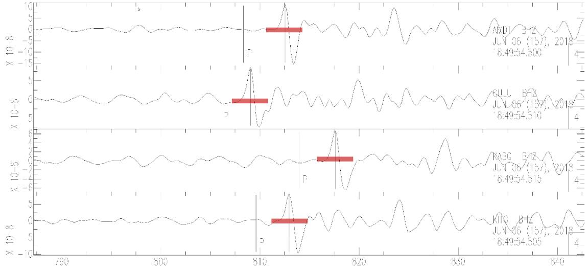
**Figure 2-4:** Example of filtered P-wave recorded on NE Uganda AfricaArray Network stations. The P-marker designates the predicted arrival using the IASPI91 model. The unlabeled marker indicates the manual pick. The red bar shows the 3 second window that is used in the cross-correlation.
