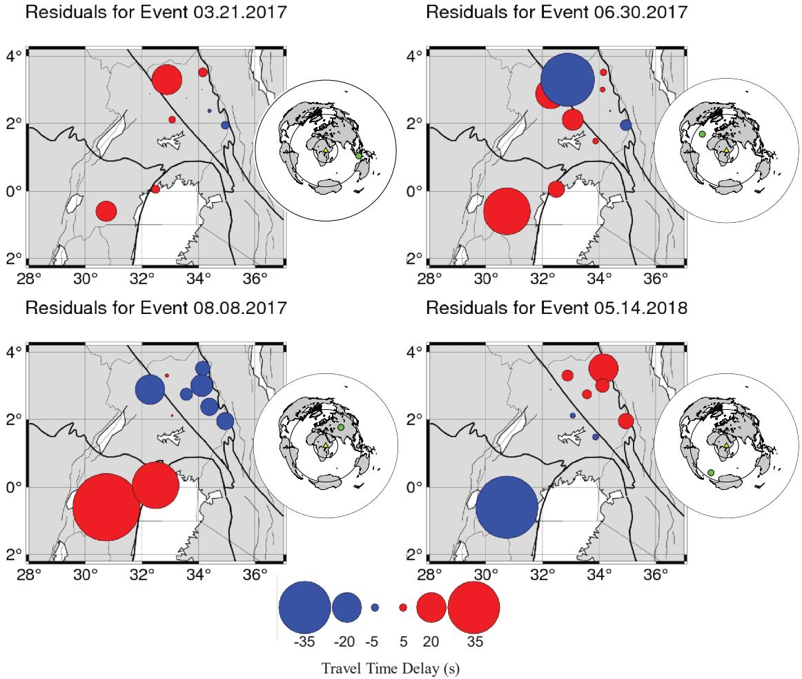
Figure 3-2: S-wave delay times for four events from 2017-2018. Inset map shows the location of the event (green dot). Circles are shown at distances of  $30^\circ$  and  $85^\circ$  away from the center of the network to indicate the range of teleseismic events. Geology is from *Katumwehe et al. [2016]* and *Mulibo and Nyblade [2013]*.
