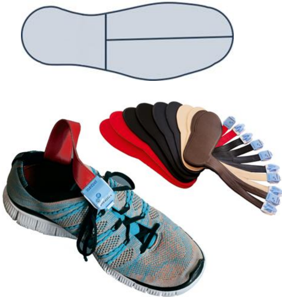
Figure 3-2 Force-measuring insoles and sensor regions
