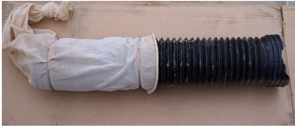
Figure 4.2: Each seed trap consisted of 10 cm of plastic pipe and 91 cm of drain sock secured with 2 rubber bands. Approximately 45 cm of sock was permitted to hang off of the trap and was tied at the loose end.
