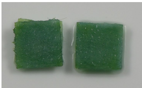
Figure S3-4. Detection of pH value for the volunteer's urine sample. Two pH stripes were used in the test and the pH values were estimated by the comparison with the reference color chart.
