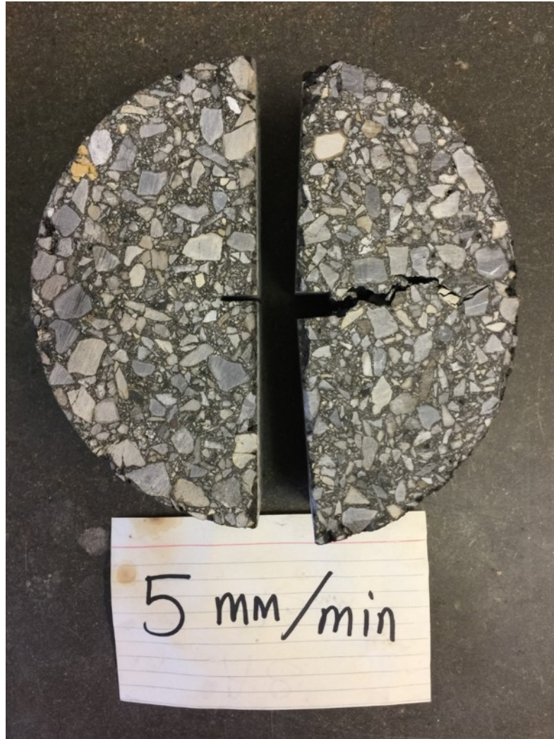
Figure 3-2. A SCB specimen before (left) and after (right) test, demonstration of a crack propagation.
