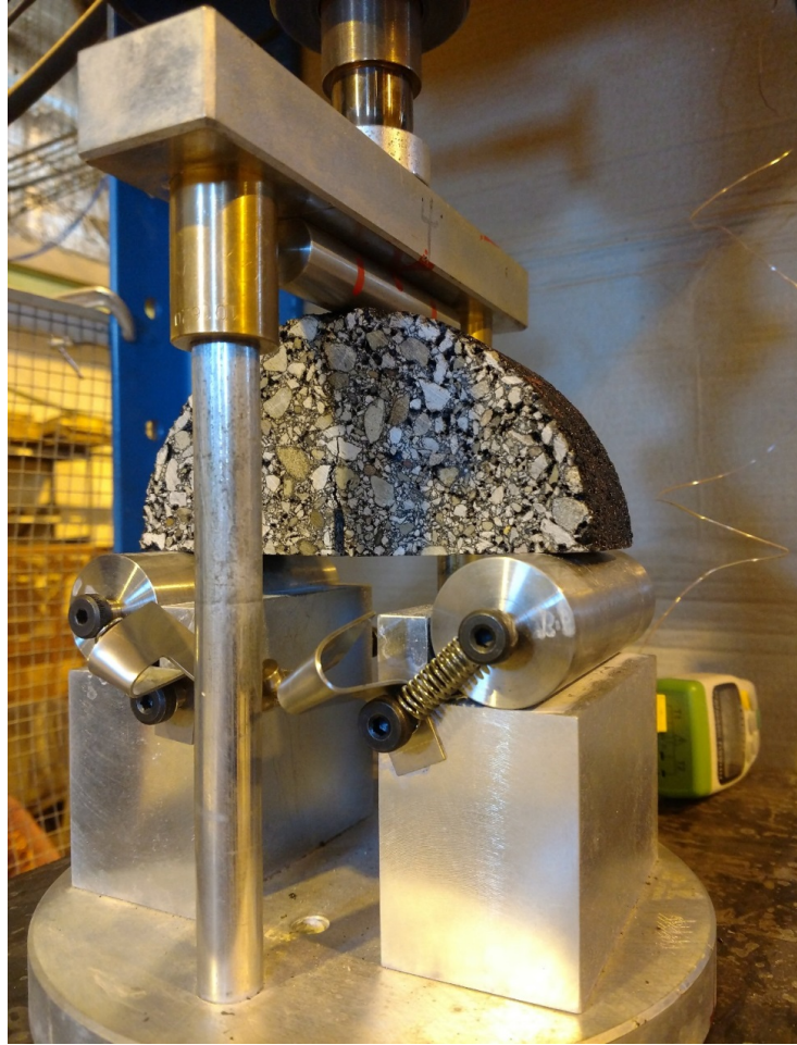
Figure 3-3. A SCB specimen after test (crack at the center of specimen).
