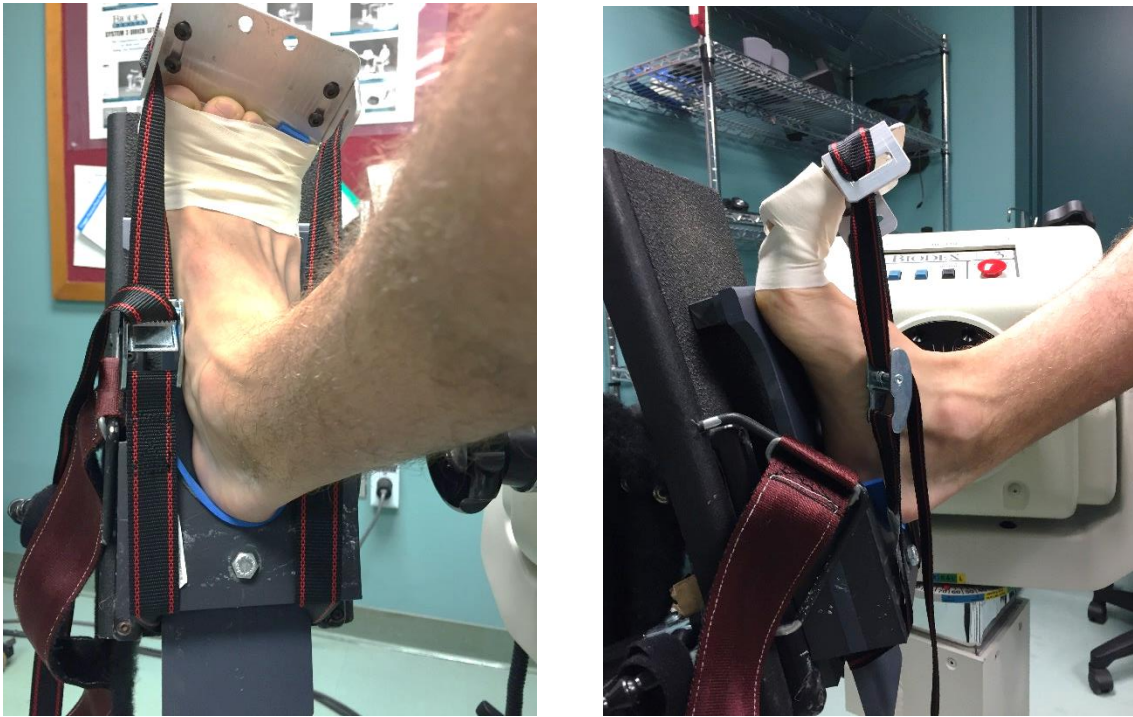
Figure 5-1 Two views of the setup used to alter MTP joint angle and remove the potential effect of the toe forces. A partial foot plate was bolted on top of the dynamometer foot plate and an aluminum toe plate with a nylon strap was used to hold the MTP joint angle during testing.
