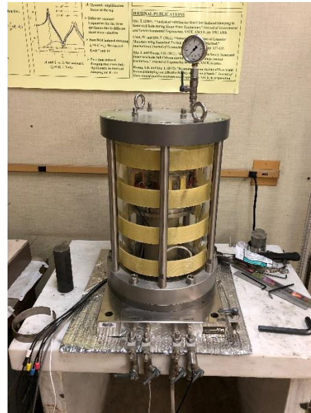
(b) Pressure chamber installed
