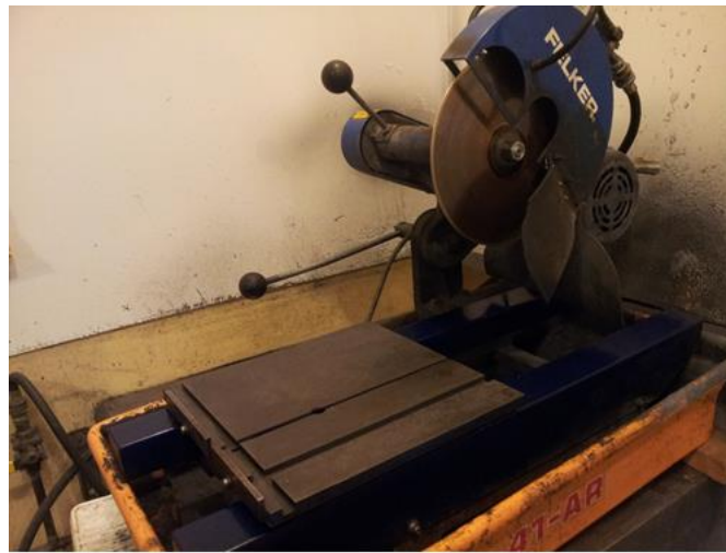
Figure 2-15: Felker 41AR 1 hp water-cooled tile saw with a diamond blade.
