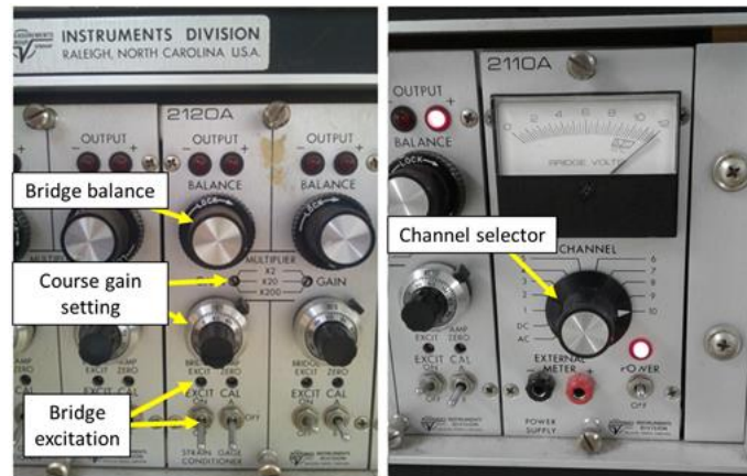
Figure 3-9: Bridge/amplifier (left), Power supply (right)
