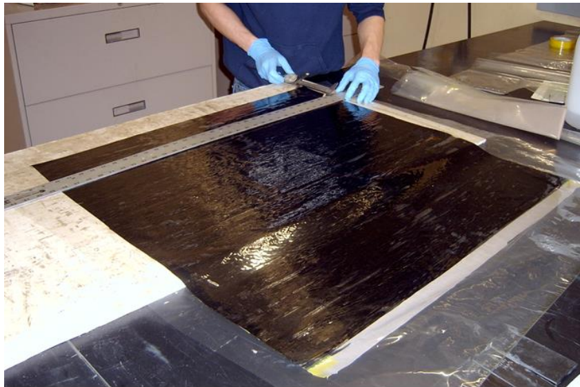
Figure 2-8: Prepreg covered with vacuum bag.
