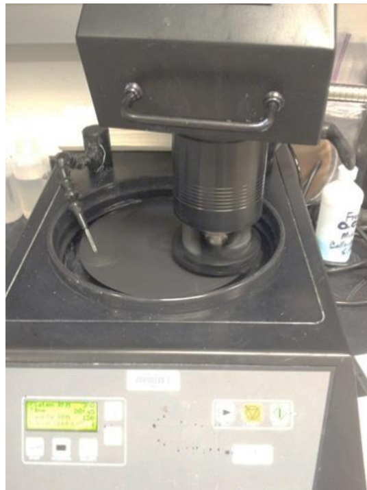
Figure 2-19: MetPrep 3™ Grinding/polishing setup.
