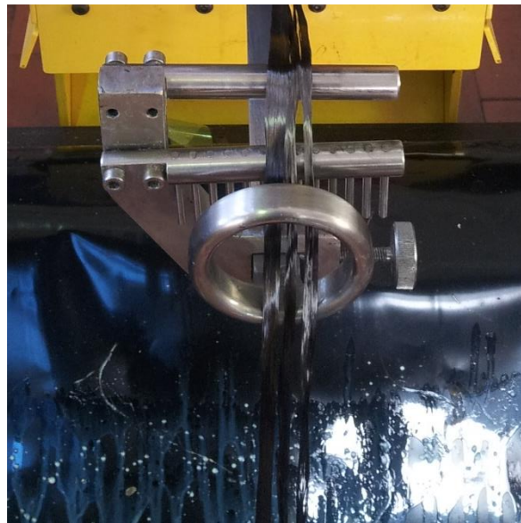
Figure 2-5: Payout eye used during the fabrication process to control the movement of the tow and to impregnate the tow with resin.
