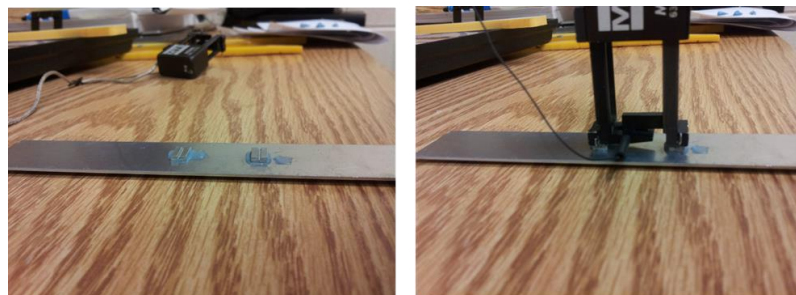
Figure 3-7: Bonding extensometer tabs (left) and aligning the tabs with the extensometer (right).
