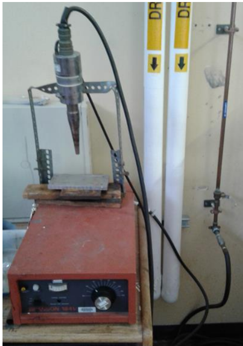
Figure 2-3: Branson 184 V 900 W 20 kHz tip sonicator.
