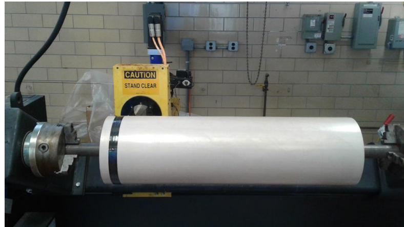
Figure 2-4: Wet filament winding carbon tow onto a round mandrel to make prepreg. McClean Anderson winding machine.
