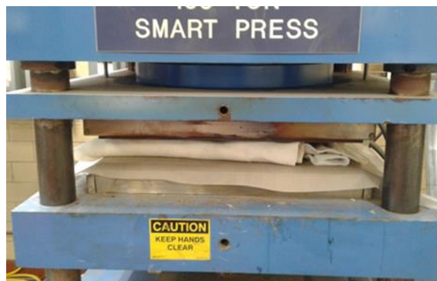
Figure 2-14: Hot pressing the two-part mold.
