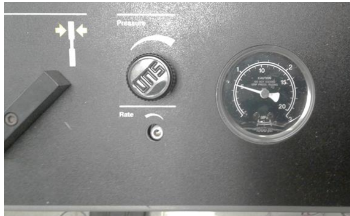
Figure 3-15: Pressure gauge of the MTS machine at 5 MPa.
