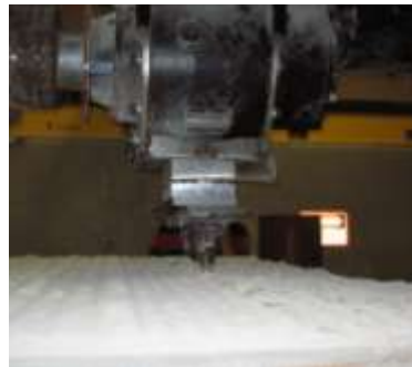
Figure 3-5 Picture of rock surface with different cut spacing during the linear cutting tests (Kim et al., 2009)
