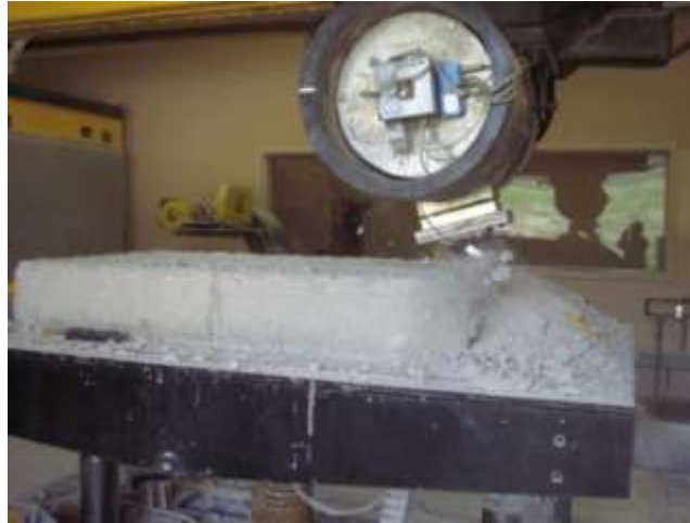
Figure 5-2 Picture of rotary cutting tests using a single bit on the cutting drum
