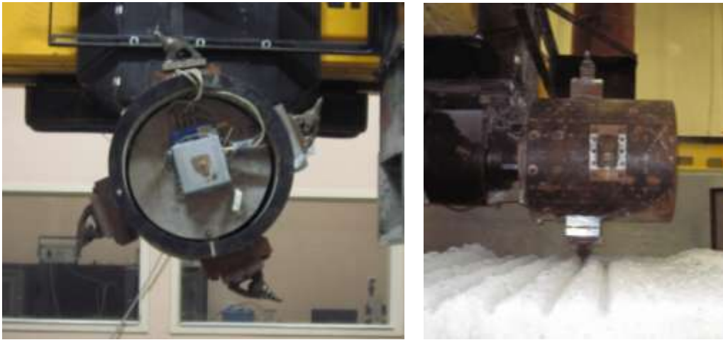
Figure 5-22 Pictures of multiple bit cutting drum lacing for rotary cutting test: (a) side view (b) front view
