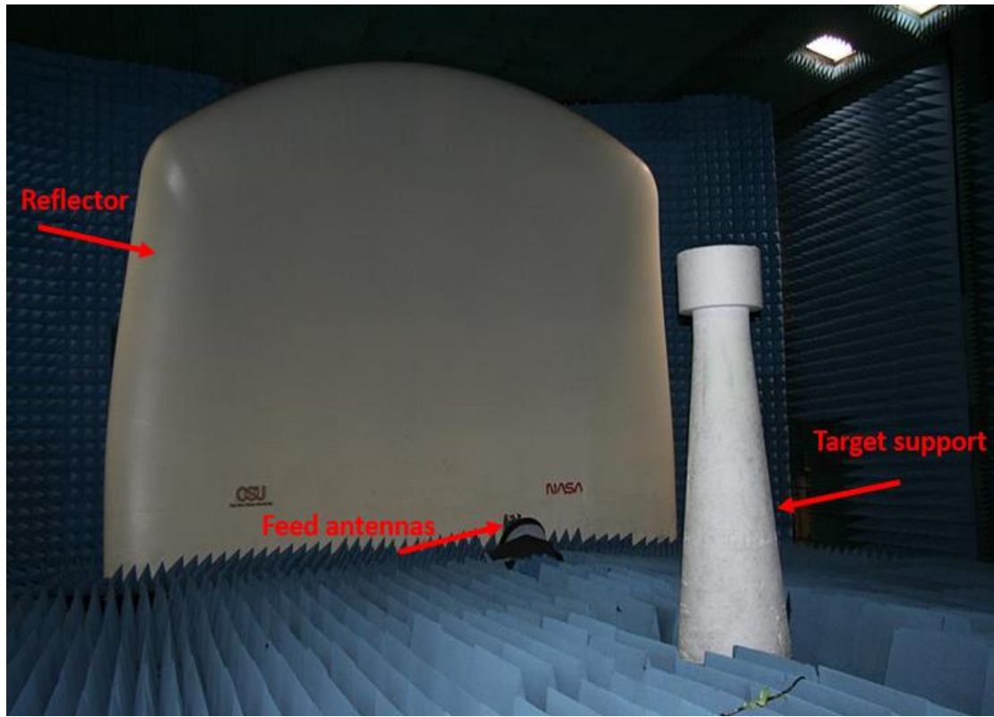
Figure 4.1: Photograph of compact radar range at ElectroScience Laboratory at The Ohio State University.
