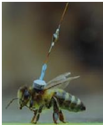
Figure 1.2: A Honeybee wearing a vertical wire transponder placed inside a detachable glass tube [23].
