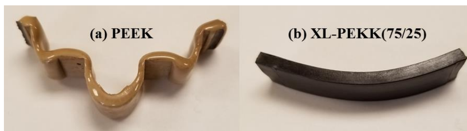
Figure 3-10: DMA specimens of (a) PEEK and (b) XL-PEKK(75/25) after temperature ramp to 400°C.
