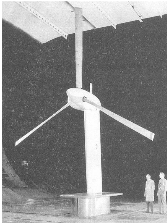
Figure 1.14: Bell Model 300 rotor in the Ames 40- by 80-ft wind tunnel (from Ref. 10)
