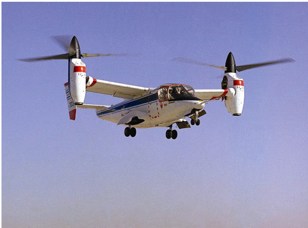
Figure 1.16: XV-15 Tiltrotor Research Aircraft in hover
